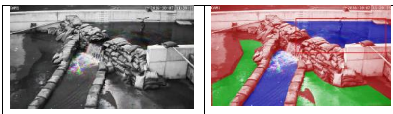
Figure 1: CCTV footage frame of flooding (left), and manually segmented image (right).
