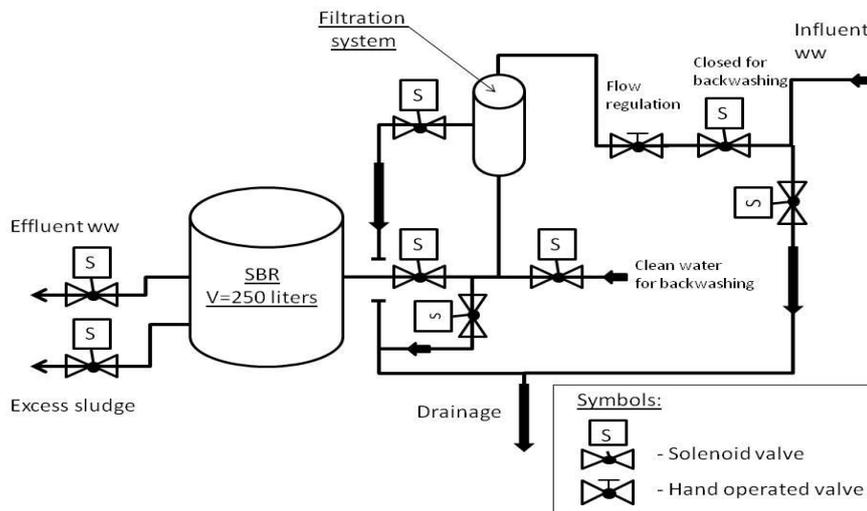
**Figure 1. Principal scheme of the treatment system with the filtration system.**
