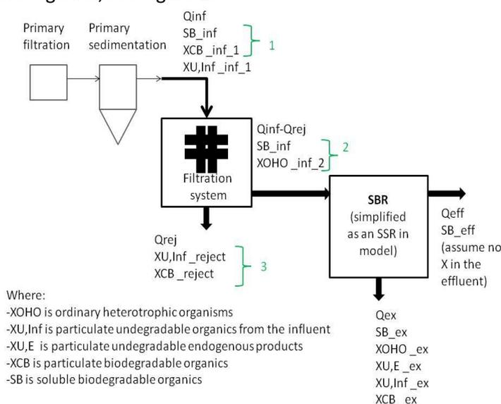
Figure 2. Flow diagram of the of the treatment system and the associated relevant variables.
