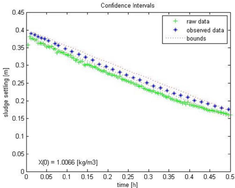
**FIGURE 5 : SLUDGE SETTLING CURVE OF RAW COMPUTED DATA VERSUS OBSERVED DATA WITH ITS CONFIDENCE BOUNDS OF 95 %. SLUDGE FROM TANK 1, STANDARD SET-UP**
