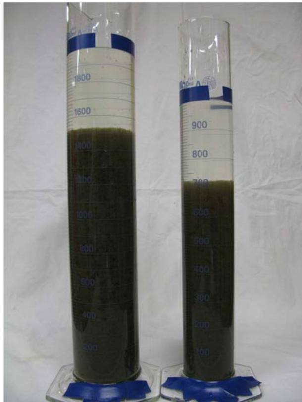
Picture: Standard set-up of Sludge Volume Experiment
