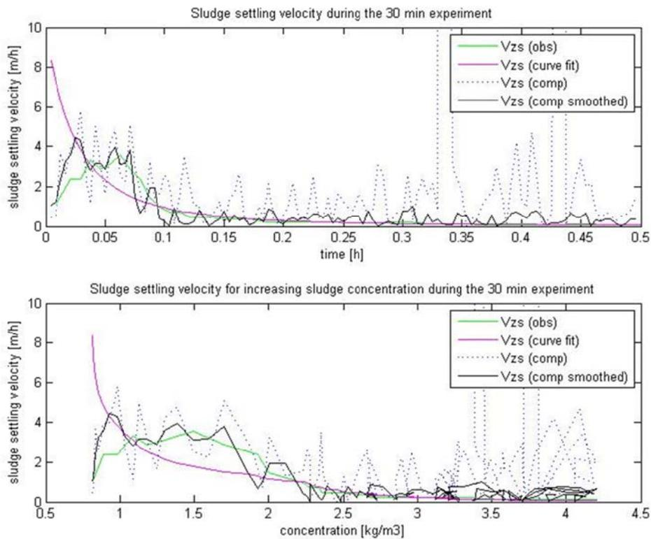
**FIGURE 11 : TRACKED SLUDGE SETTLING VELOCITY DURING THE 30 MIN SETTLING EXPERIMENT AND DURING CHANGING CONCENTRATION CONDITIONS. SLUDGE TANK 2, CAMERA ON LADDER**
