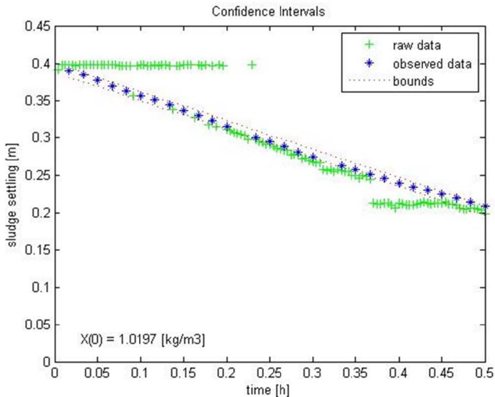
**FIGURE 6 : SLUDGE SETTLING CURVE OF RAW COMPUTED DATA VERSUS OBSERVED DATA WITH ITS CONFIDENCE BOUNDS OF 95 %. SLUDGE FROM TANK 1, FLASH**
