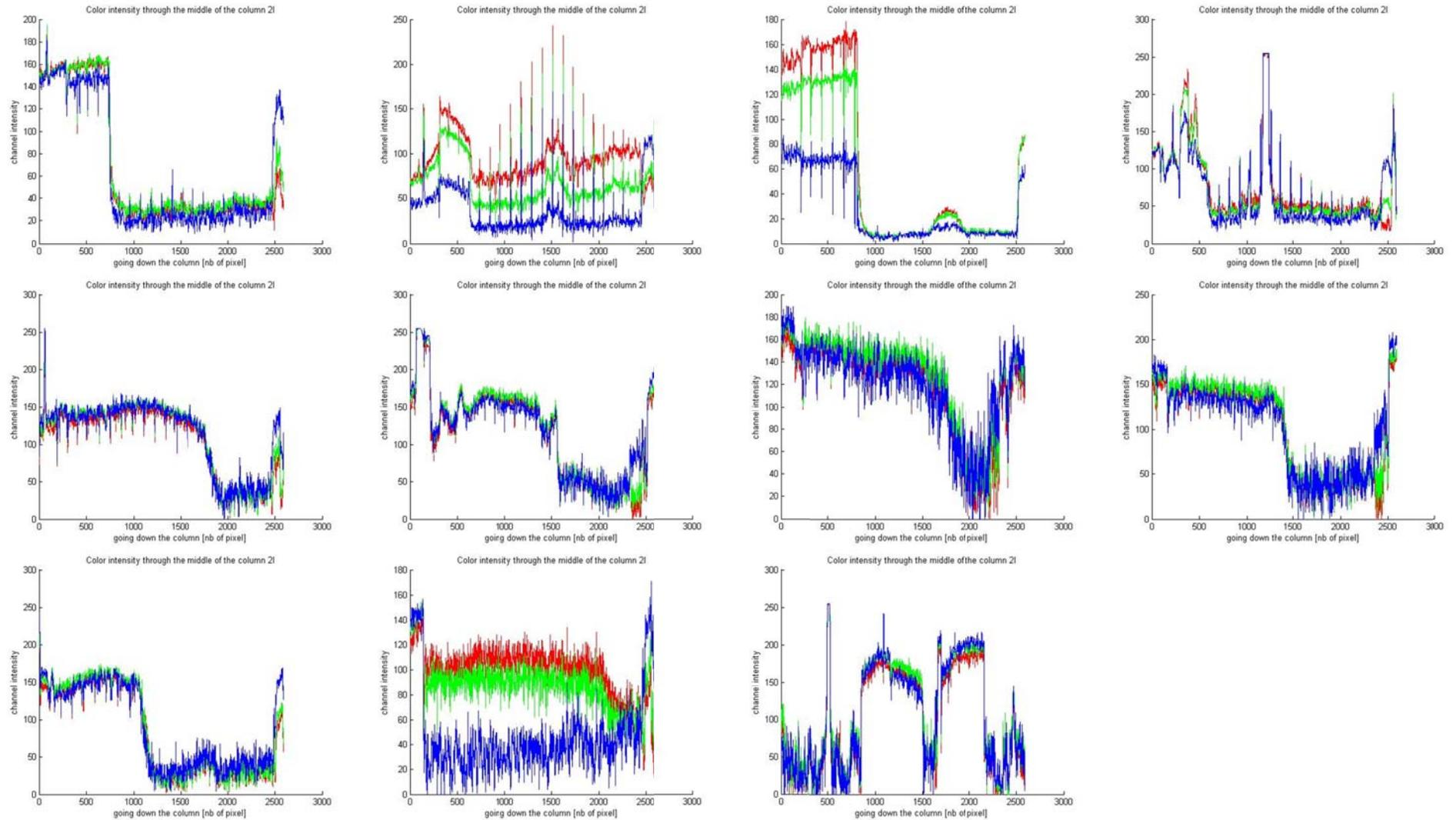
**TABLE 10: OVERVIEW OF THE SIMULATION RESULTS COMPARED TO THE OBSERVED DATA COLUMN** (FIRST LINE: SLUDGE TANK 1; STANDARD, FRONT FLOOD LIGHT, BACK FLOOD LIGHT, FLASH. SECOND LINE: SLUDGE TANK 2; STANDARD, CAMERA ON TABLE, CAMERA ON LADDER, CAMERA AT 2.3 M WITH ZOOM. THIRD LINE: STANDARD SETTING FOR SLUDGE WWTP WINTERTHUR, URIN TANK)
