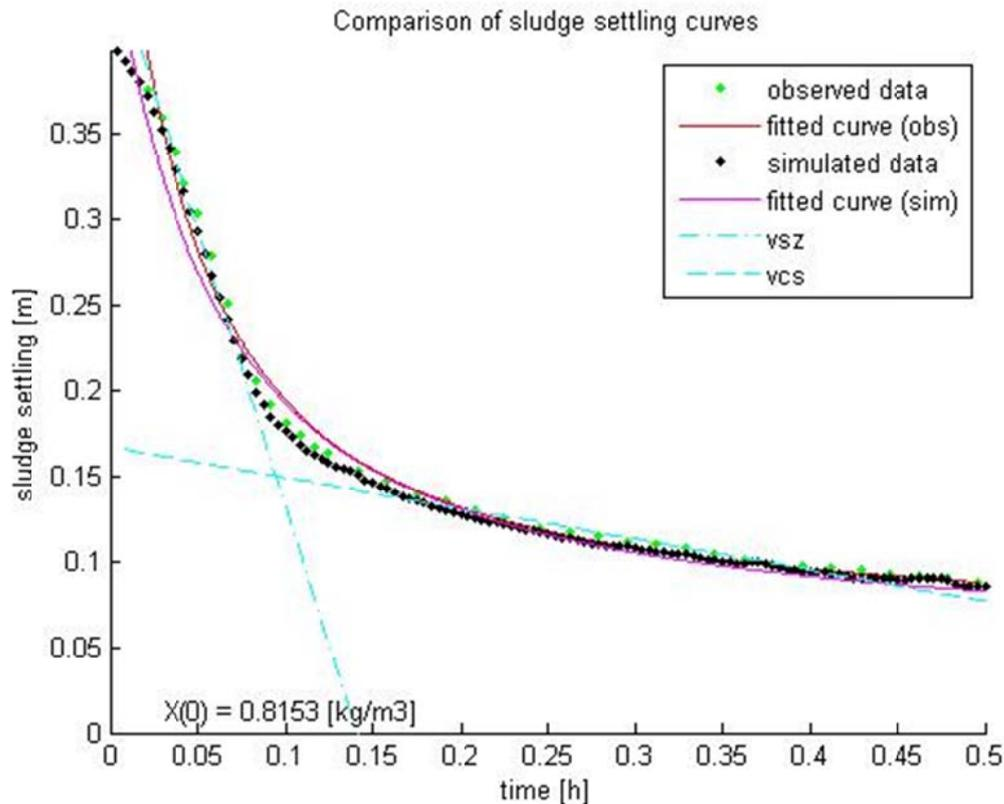
**FIGURE 9 : SLUDGE SETTLING CURVE OF THE OBSERVED DATA, THE FILTERED RAW DATA AND THEIR EXPONENTIAL CURVE FIT. ESTIMATED ZONE SETTLING VELOCITY (VSZ) AND COMPRESSION SETTLING VELOCITY (VCS) ARE DETECTED. SLUDGE FROM TANK 2, CAMERA AT 2.3 M, ZOOM**
