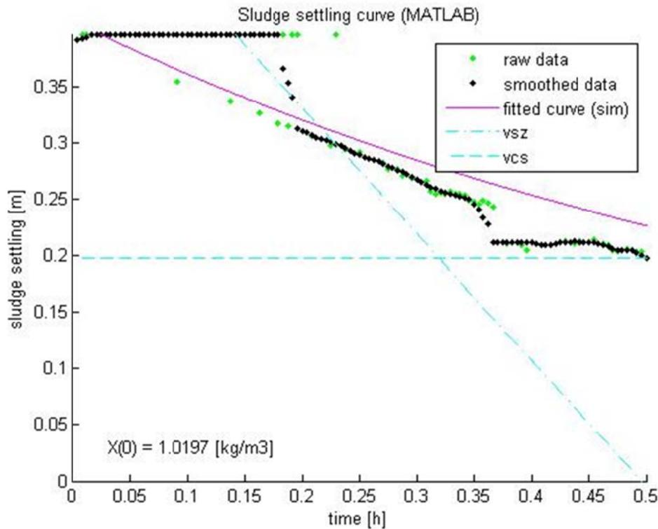
**FIGURE 7 : SLUDGE SETTLING CURVE OF RAW COMPUTED DATA AND THE FILTERED RAW DATA AND THE EXPONENTIAL CURVE FIT. ESTIMATED ZONE SETTLING VELOCITY (VSZ) AND COMPRESSION SETTLING VELOCITY (VCS) ARE DETECTED. SLUDGE FROM TANK 2, FLASH**
