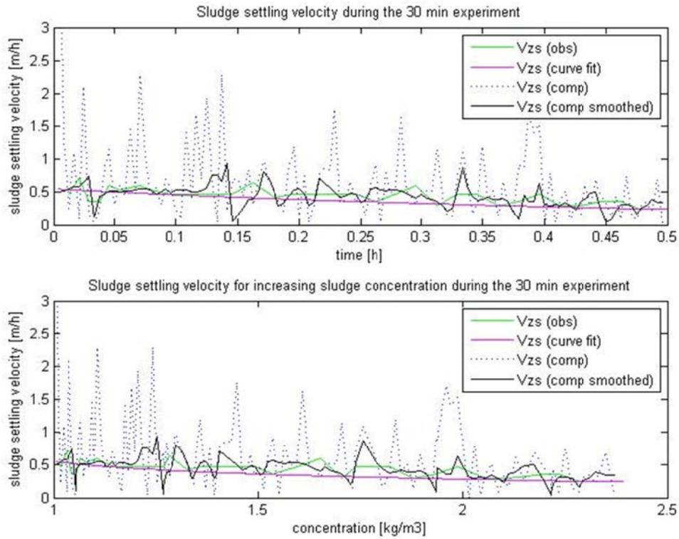
**FIGURE 10 : TRACKED SLUDGE SETTLING VELOCITY DURING THE 30 MIN SETTLING EXPERIMENT AND DURING CHANGING CONCENTRATION CONDITIONS. SLUDGE TANK 1, STANDARD SET-UP**
