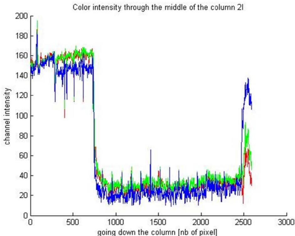
**FIGURE 3 : RED GREEN BLUE CHANNEL INTENSITY ANALYSIS OF SLUDGE FROM TANK 1 THROUGH THE MIDDLE OF THE COLUMN 2L WITH SLUDGE FROM TANK 1 AND STANDARD SET-UP**
