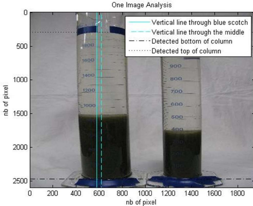
FIGURE 4 : VERTICAL LINES THROUGH THE 2L SLUDGE COLUMN SERVING TO DETECT THE BOTTOM AND THE TOP OF THE GRADUATION OF THE COLUMN WITH SLUDGE FROM TANK 1 AND STANDARD SET-UP.
