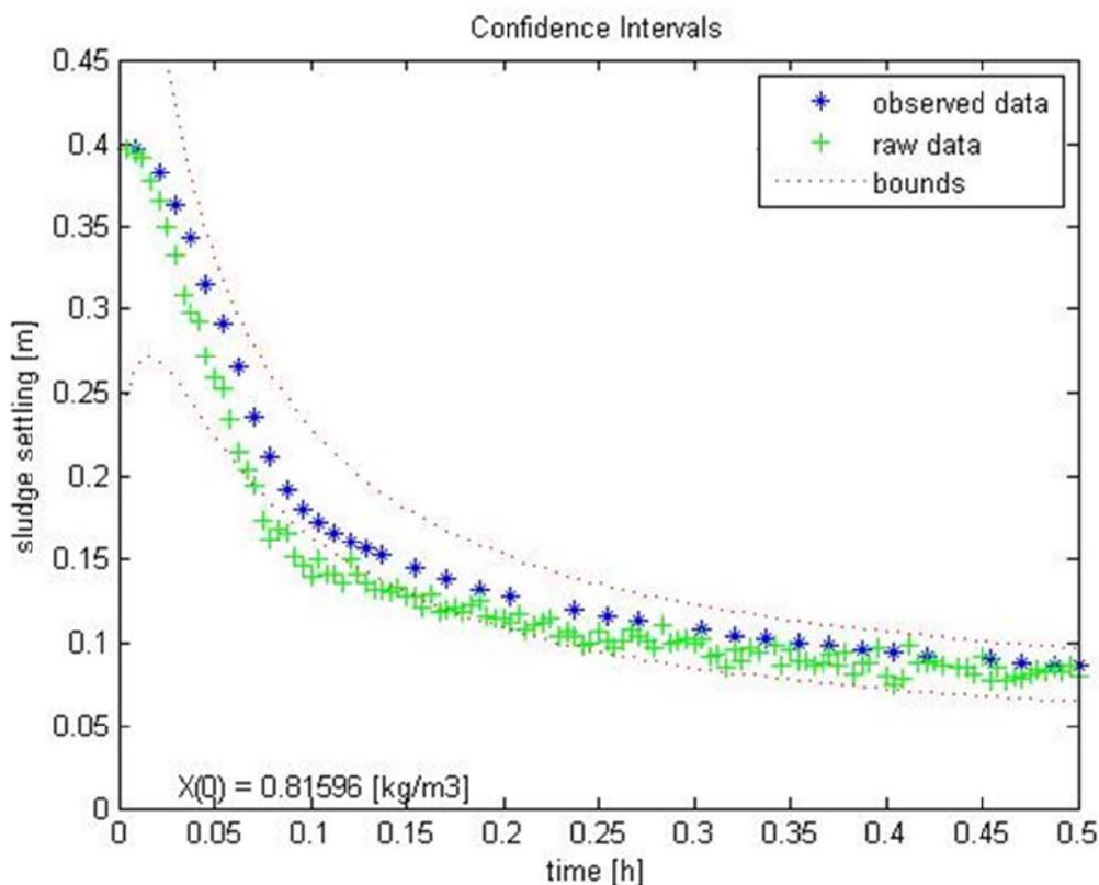
**FIGURE 8 : SLUDGE SETTLING CURVE OF RAW COMPUTED DATA VERSUS OBSERVED DATA WITH ITS CONFIDENCE BOUNDS OF 95 %. SLUDGE FROM TANK 2, CAMERA ON LADDER**
