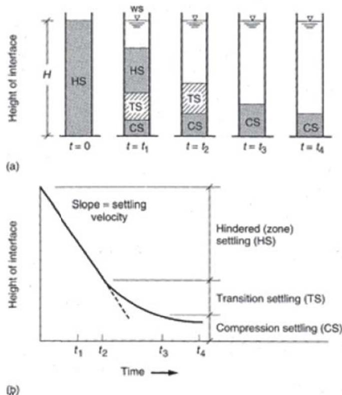
FIGURE 1 : DEFINITION SCETCH FOR HINDERED (ZONE) SETTLING: (A) SETTLING COLUMN IN WHICH THE SUSPENSION IS TRANSITIONING THROUGH VARIOUS PHASES OF SETTLING AND (B) THE CORRESPONDING INTERFACE SETTLING CURVE (SOURCE: METCALF AND EDDY [10])
