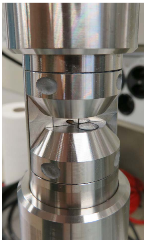
Figure 2: Sensor window in measuring gap of UV-Vis spectrophotometer.
