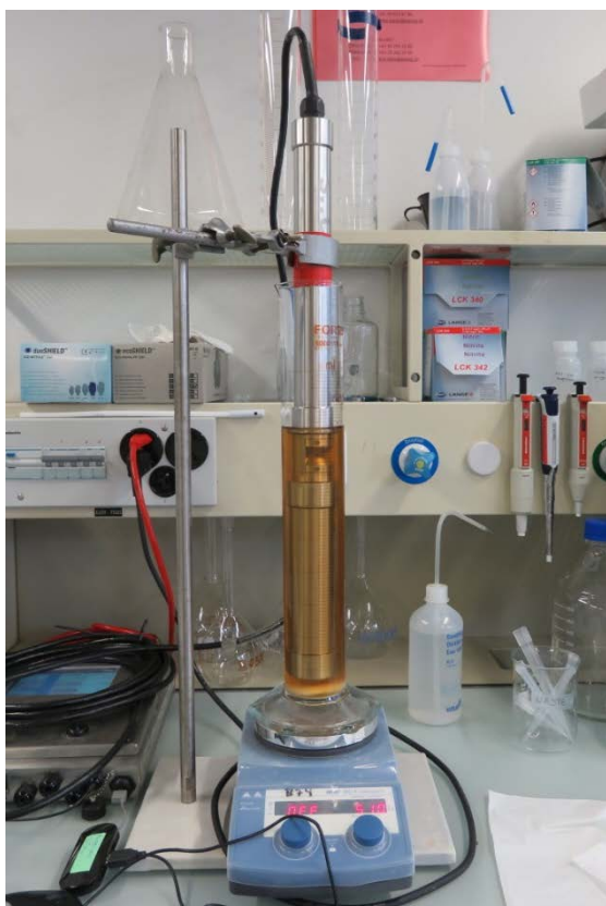
Figure 1: UV-Vis spectrophotometer recording absorbance spectra in a urine sample.
