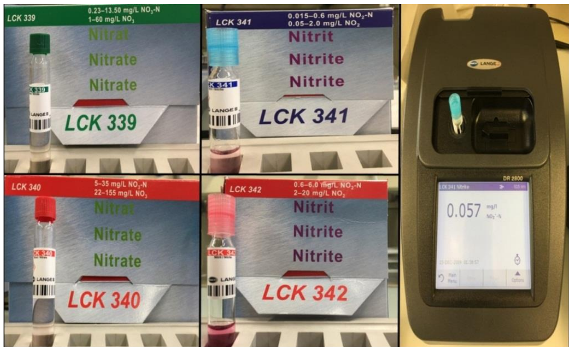
Fig 8.1: Images of Hach-Lange cuvette and Hach DR 2800 spectrophotometer
