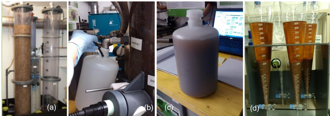
Figure 3.4. Sample Collection and Decantation steps: (a) Nitrification reactor; (b) Urine sampling (c) Urine plastic container; (d) Imhoff cones
