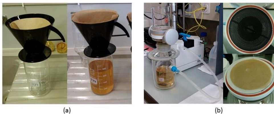
Figure 3.7. Sample Filtration: (a) Coffee filtration and (b) Microfiltration
