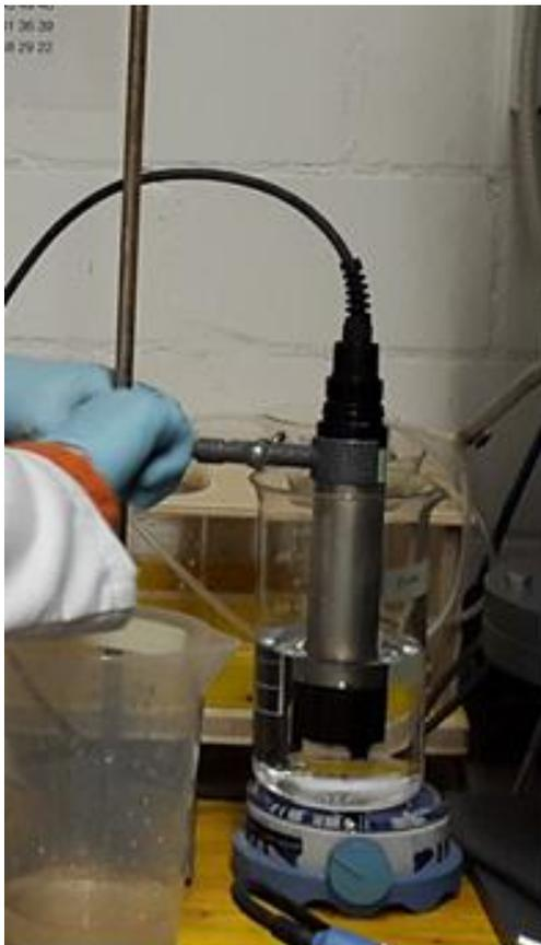
**Figure 5. DO sensor setup with efficient mixing, here for saturated nanopure water.**
