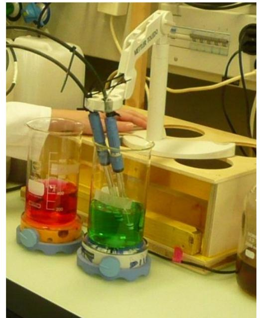
**Figure 7. Experimental setup with 2 pH sensors for pH 7 and pH 4 buffer solutions.**
