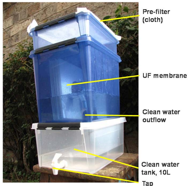
Figure 10 GDM filter prototype \alpha -version for the field study in Kenya (photo: S. Derksen, M. Peter)
