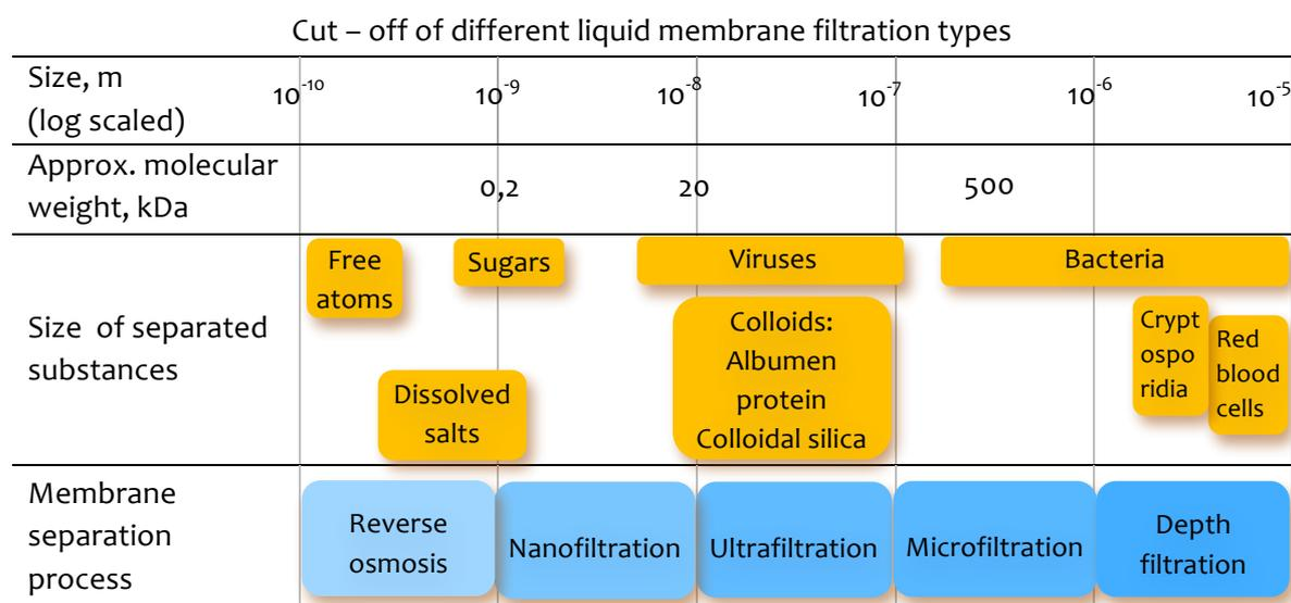
**Figure 1** Overview of membrane pore sizes, removed contaminants and the applications (AWWA 2005).
