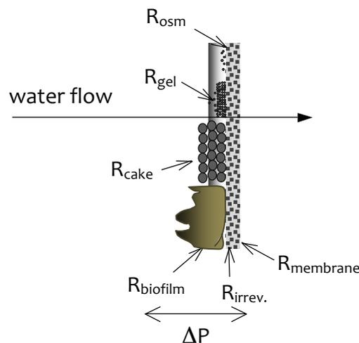
**Figure 2** Partial resistances during membrane filtration that lead to transmembrane pressure loss  $\Delta P$ .
