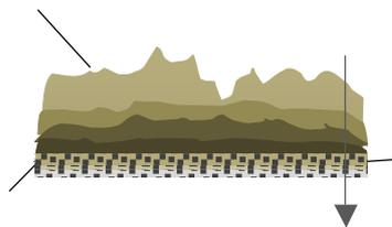
**Figure 1** Stratification and heterogeneity of the biofilm layers and of the resistances to filtration. The darker colour biofilm means higher resistance, with least resistive layers further away from the membrane surface. EPS sorption into the membrane pores itself cannot be excluded from estimating resistances to filtration.
