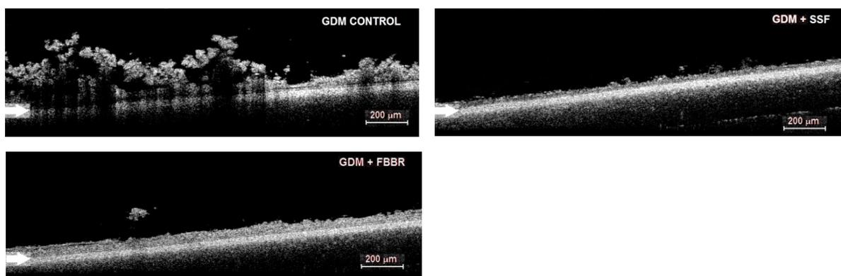
**Figure 4** Thickness of the biofilm formed on the membrane surface for each system, imaged by OCT (day 76). GDM control - without pre-treatment; GDM+PBBR - GDM with packed bed bioreactor; GDM+SSF – GDM with slow sand filter. The white arrows indicate the membrane surface.
