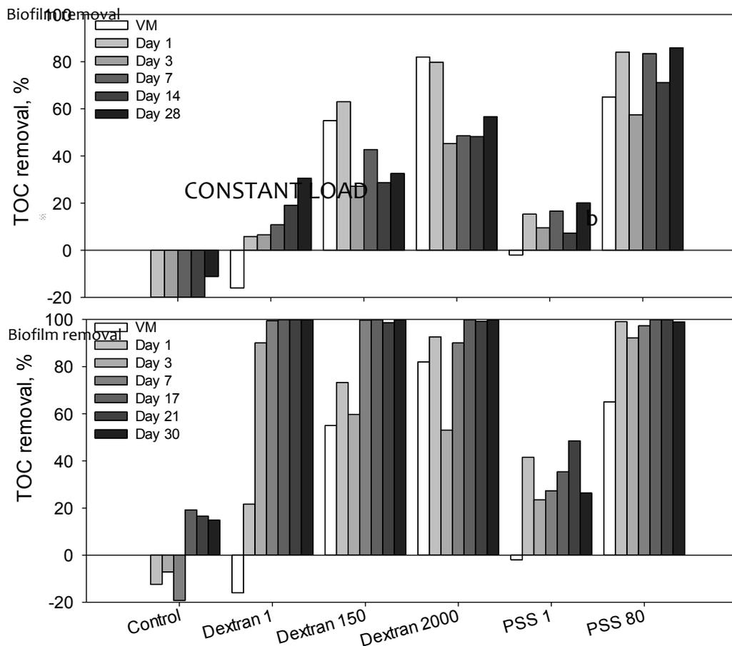
**Figure 2** Permeate quality for Exp. A and B, based on retention and degradation of foulants (TOC measurements). Each error bar indicates a standard deviation. a – variable load experiment, b – constant load. The retentions are compared to the virgin membrane retention (VM) and retention after the biofilm was removed from the membrane surface, at the end of experiment (indicated by the dashed line - - - -).
