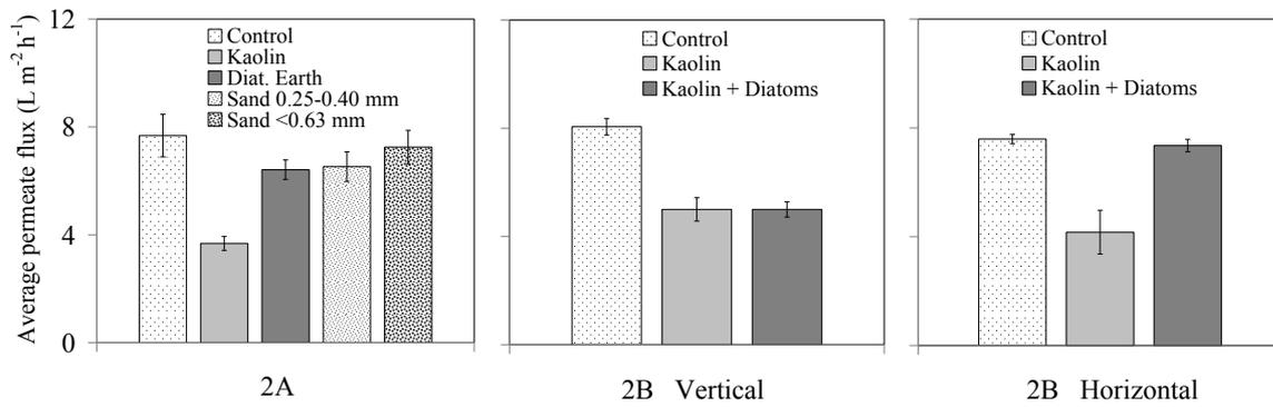
**Figure 6** Permeate flux values from the flux stable period of the particle pre-coated membranes (2A) during dead-end filtration of creek river water, compared to continuous particle addition filtration (2B), performed in two membrane configurations: horizontal and vertical. Each error bar indicates standard deviation.
