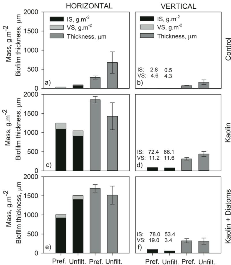
**Figure 3** Comparison of volatile (VS), inorganic (IS) solids and biofilm thickness in two membrane configurations: horizontal and vertical. One membrane filter was weighed at the end of exp. A (prefiltered), two membranes for exp. B (unfiltered creek water). For the vertical configuration numeric values for VS and IS are provided.
