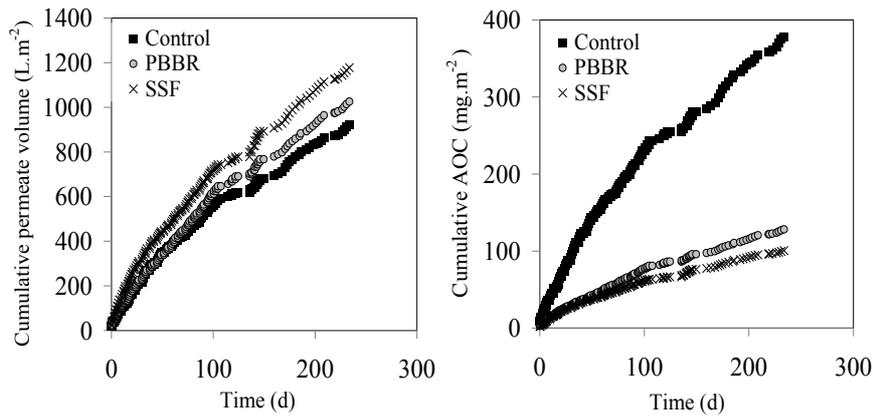
**Figure 5** Differences in permeate volumes between the three systems (A), and corresponding cumulative values of AOC reaching the membrane surface (B) for: control - GDM (without pre-treatment) PBBR – GDM with packed bed bioreactor as pre-treatment; SSF – GDM with slow sand filter as pre-treatment.
