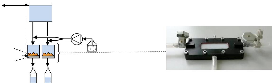
**Figure 1** Experimental setup with addition point of the foulants - dextrans or polystyrene sulfonates (left), and the biofouling monitor (right). Each experimental line consisted of two biofouling monitors fed from a daily prepared, autoclaved creek water solution. No foulant was added to control. Six identical experimental lines were used in parallel for both experiments A and B.
