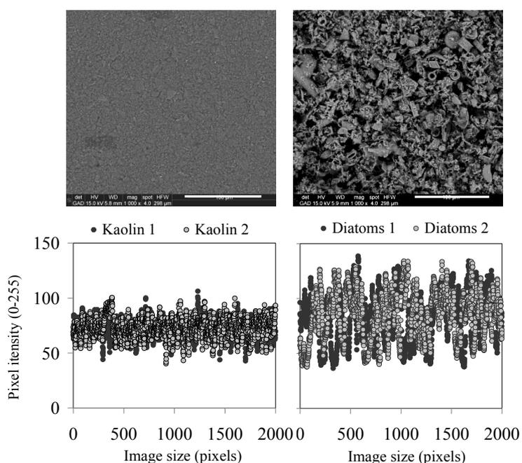
**Figure 7** Top view SEM micrographs of biofilm structure formed in the presence of kaolin (A) and diatomaceous earth (B), from Experiment 2A. Image size area 300 x 300  $\mu\text{m}$ .
