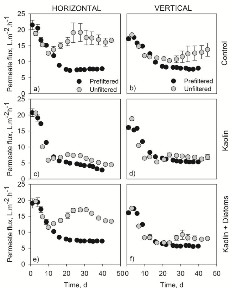
**Figure 2** Permeate flux values obtained during continuous dead-end filtration of creek water, spiked with kaolin or kaolin with diatomaceous earth (50/50%), compared to control (no particle addition), in two membrane configurations: horizontal and vertical. Each error bar indicates standard deviation.
