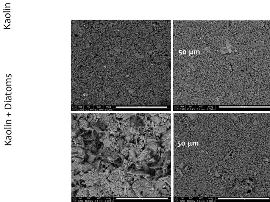
**Figure 4** Scanning Electron Microscopy micrographs of the deposited biofilm layers (in top view) demonstrate effects of particle selection in horizontally (A, C) and vertically (B, D) oriented membranes (experiment A). Membranes were fed with the same raw water, spiked with  $300 \text{ mg L}^{-1}$  kaolin (A, B) or  $300 \text{ mg L}^{-1}$  kaolin and diatoms (C, D) (50/50%, by weight). Image size area  $100 \times 100 \text{ }\mu\text{m}$ .
