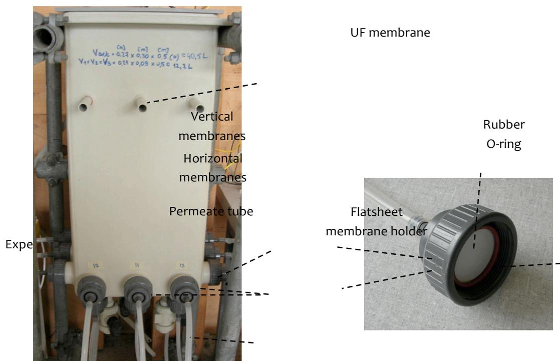
**Figure S1** Photograph of the experimental tank and the flatsheet membrane holder.
