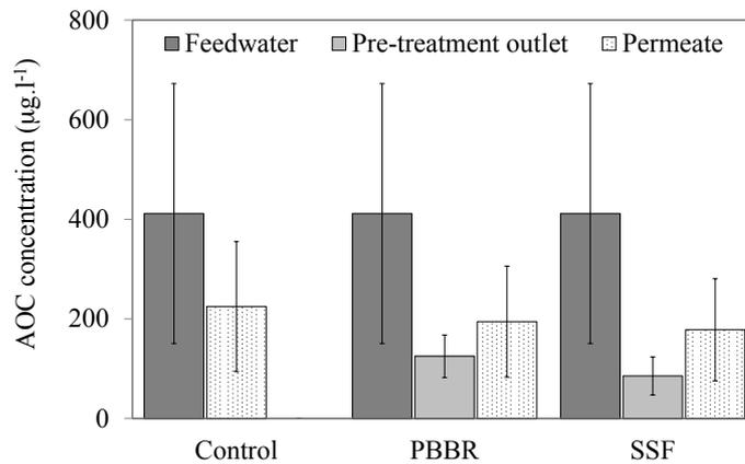
**Figure 3** Mean AOC concentrations of the three systems studied: control – GDM with creek river water without pre-treatment; PBBR – GDM with packed bed bioreactor as pre-treatment; SSF – GDM with slow sand filter as pre-treatment.
