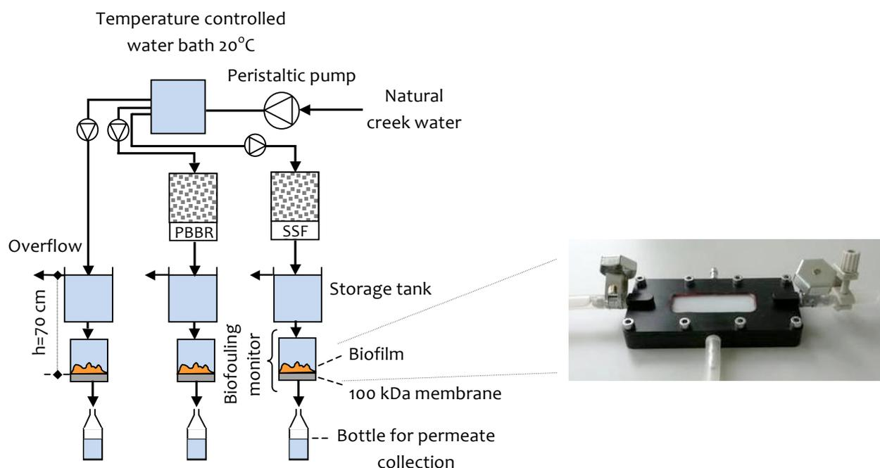
**Figure 1** Schematic layout of the Experiment 1 setup (left) with the biofouling monitor (right).
