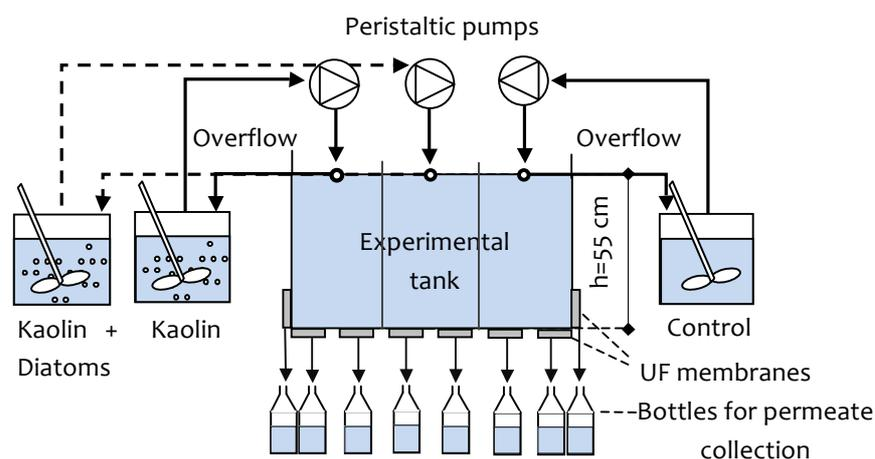
**Figure 2** Schematic layout of the Experiment 2 setup.
