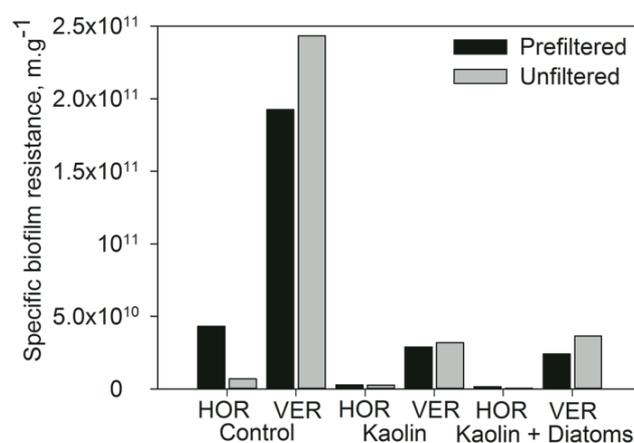
**Figure 5** Specific biofilm resistance from experiment A and B, obtained by division of the biofilm resistance ( $R_{\text{biofilm}}$ ) with its corresponding total solids (TS) mass.
