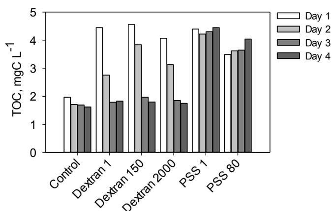
**Figure S1** Foulant degradation in a batch experiment. The foulants were added to continuously stirred, thermostated at 20°C glass vessels filled with 1 L prefiltered (0.4 µm) creek water. A TOC sample was taken and analyzed every day. TOC level in control is from creek water, as no foulant was added.
