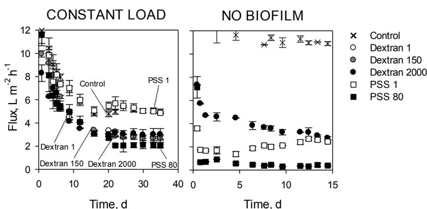
**Figure 4** Permeate flux for constant load (Exp. B), compared to flux without biofilm (Exp. C). Exp. B was conducted in prepared creek water, with  $7 \text{ mg L}^{-1}$  foulants added as product, while exp. C was conducted in deionised water, with  $50 \text{ mg L}^{-1}$  foulants added as product ( $25 \text{ mg L}^{-1}$  as organic carbon). Each error bar indicates a standard deviation.
