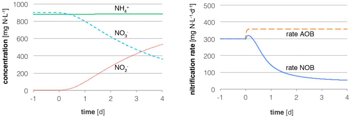
**Figure 3:** Simulation of nitrite accumulation (left) and corresponding AOB and NOB activity (right) caused by a sudden increase of the influent rate by a factor of 1.2.
