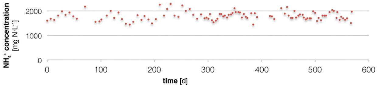
**Figure 2:** Fluctuating ammonium concentration in the reactor influent tank.
