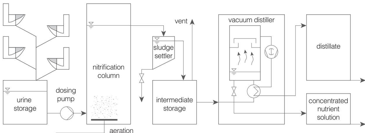
**Figure 1:** Flow diagram of the reactor set-up for total nutrient recovery from urine.
