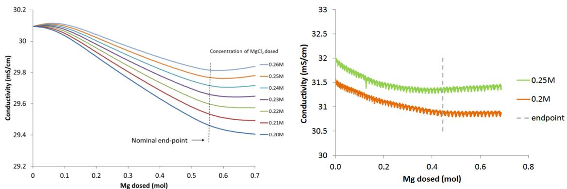
Figure 4: Modelled conductivity for different  $\text{MgCl}_2$  solutions (left) and experiments on the reactor with selected molarities (right).
