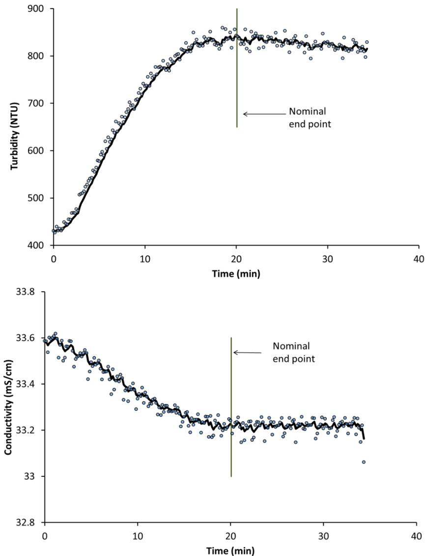
Figure 7: Conductivity and turbidity for continuous dosing of 0.5 mol/L  $\text{MgSO}_4$  at 0.73 mL/s. The dark line represents a smoothed signal, which still exhibits significant fluctuations.
