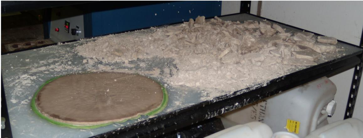
Figure 3: Struvite retained on cloth filter from 100 L urine processed and dried struvite.
