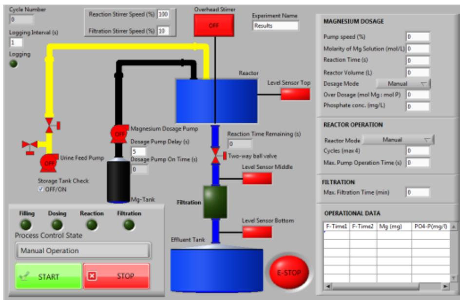
Figure 2: Software panel for reactor control programmed in LabView.
