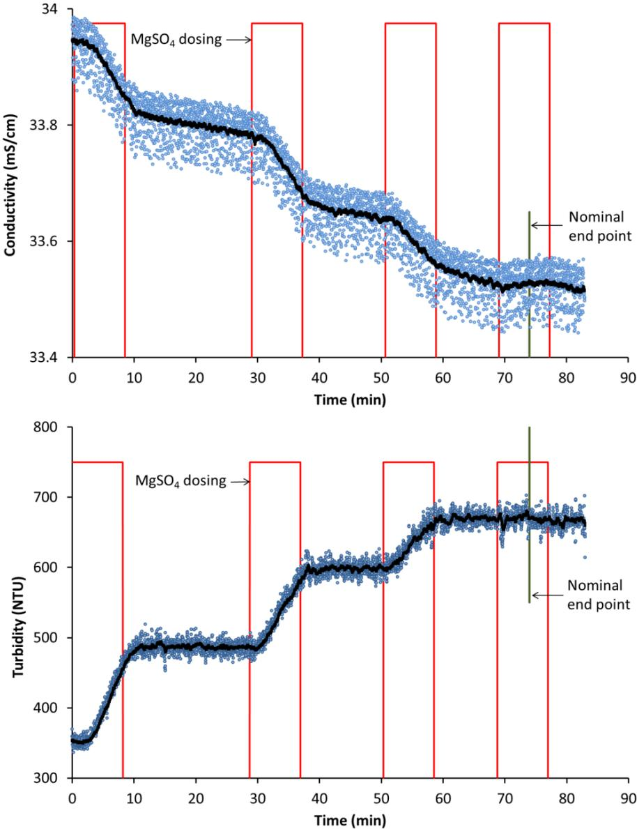
Figure 8: Conductivity and turbidity for intermittent dosing of 0.5 mol/L MgSO<sub>4</sub> at 0.73 mL/s. The dark line represents a smoothed signal. The red line indicated when the dosing pump was switched on or off.
