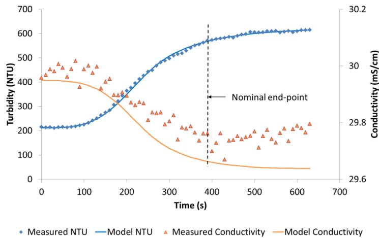
Figure 5: Measured and modelled conductivity and turbidity readings for a 0.5 mol/L  $\text{MgSO}_4$  solution added at 2 mL/s.
