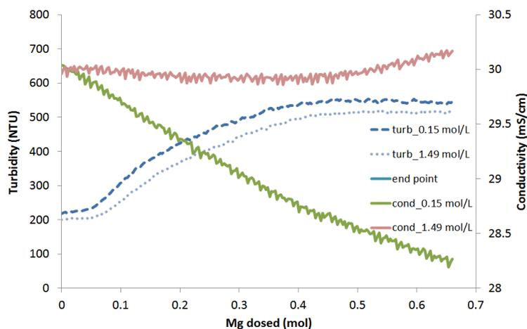
Figure 6: Conductivity and turbidity readings when switching the dosing parameters using  $\text{MgSO}_4$ , 0.15 mol/L and 2 mL/s compared to 1.49 mol/L and 0.2 mL/s while keeping the added magnesium per second (0.3 mmol/s) constant.
