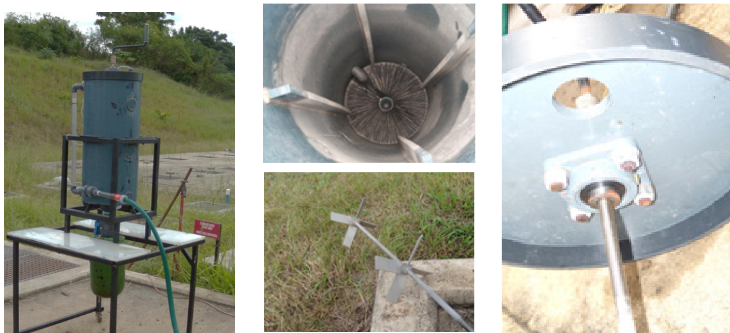
Figure 1: Simple, manually-operated struvite reactor, clockwise from left: overall assembly and placement; vertical baffles in interior; dual impellers; bearing assembly and dosing inlet port viewed from underside of cover.
