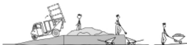
Figure 6.3: Sorting on a platform. Waste is delivered onto the platform. Workers stand upright and sort out organic waste and fill it into wheelbarrows below. Advantage: no further need for shoveling and no direct contact with the waste
