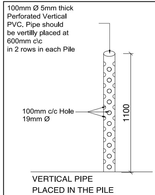
c. Bottom level drainage grid construction with PVC pipes of the compost box
