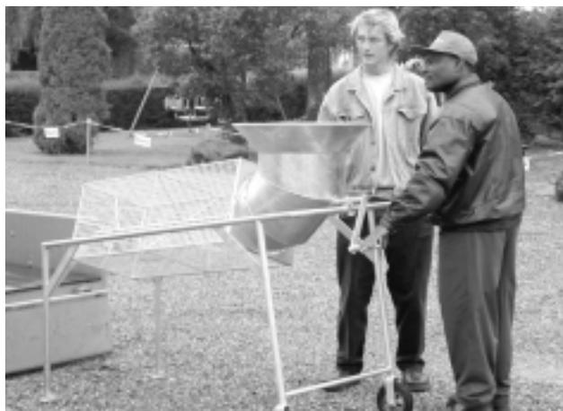
Photograph 7.15: Manual rotating drum sieve with rectangular drum (15 mm mesh size). Compost is shovelled into the hopper which is feeding the rotating drum sieve. (CompoSieb, jbsART, Switzerland)
