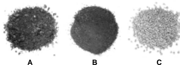
Photograph 8.1: A: Mature compost, B: ground compost and C: amended/granulated compost
