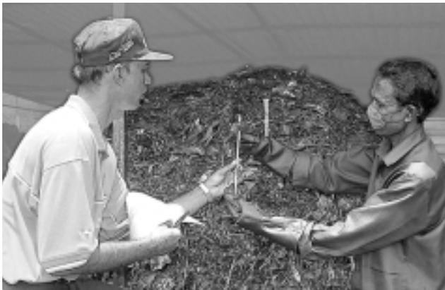
Photograph 7.9: Temperature measurement with an alcohol thermometer (Waste Concern, Bangladesh)
