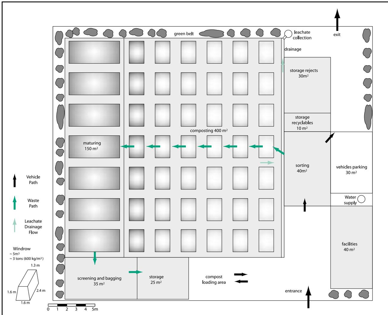
4B: a) Box-composting system, layout plan
