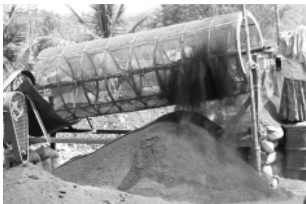
Photograph 7.16: Motor driven rotating drum sieve for larger amounts of compost (20 tons/day). (Terra Firma, India)
