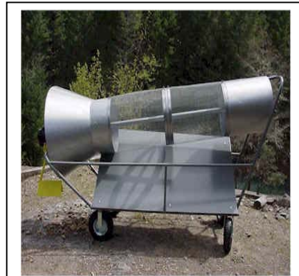
Fig 5: Small to medium-scale harvesters such as this one can be used to harvest hundreds of pounds of worms per day.
