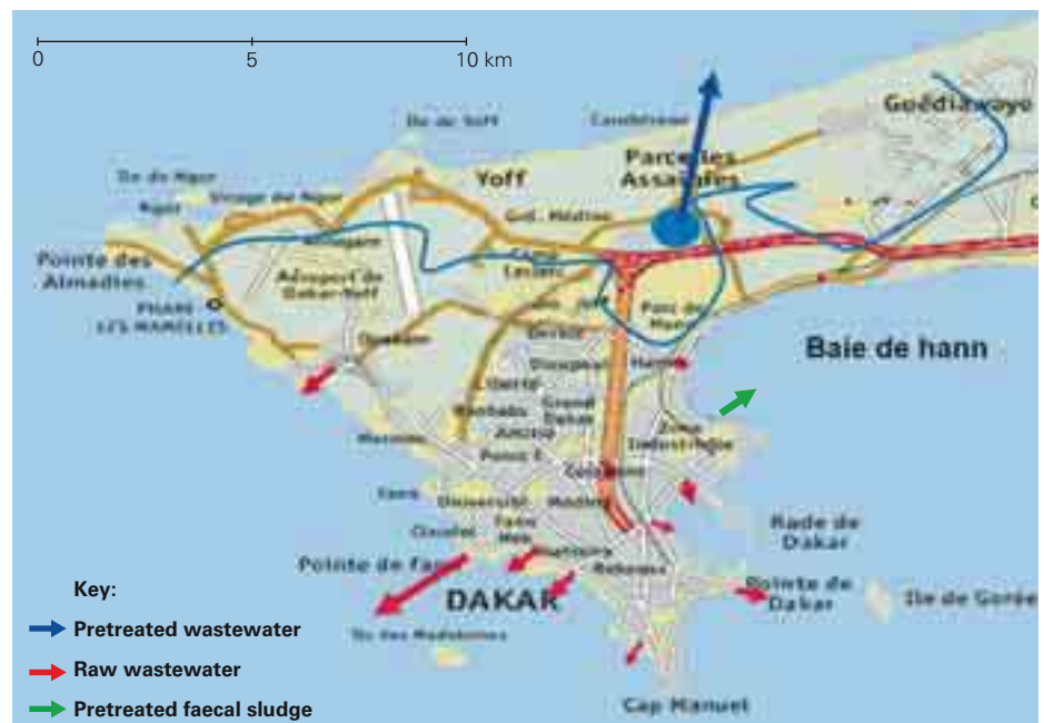
Figure 1: Overview of Dakar's faecal sludge and wastewater discharge before implementing PaqpuD, the World Bank co-financed sanitation upgrading programme.
