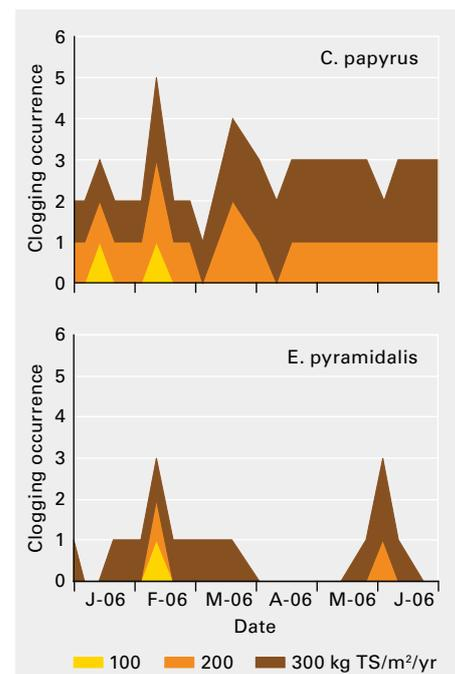
Figure 1: Occurrence of clogging events in the different beds as a function of the solid loading rates applied.
