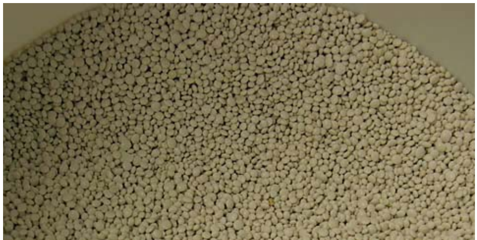
Photo 3: Ideally, the struvite will have a uniform, pellet-like shape for easy application and spreading.
