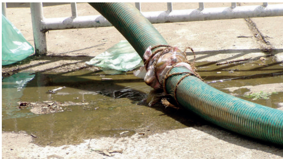
Figure 4.4 Hoses and fittings require frequent attention and repairs to keep them functioning properly. This picture illustrates inadequate maintenance, resulting in leaking of FS from the emptying hose (photo: David M. Robbins).
