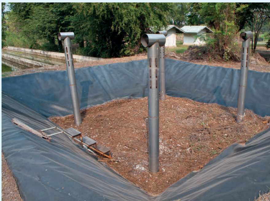
Figure 8.4 A currently out of use pilot-scale drying bed at the Asian Institute of Technology (AIT), showing ventilation pipes (photo: Linda Strande).
