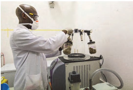
Figure 2.20 Freeze-drying of faecal sludge samples (photo: UKZN PRG).
