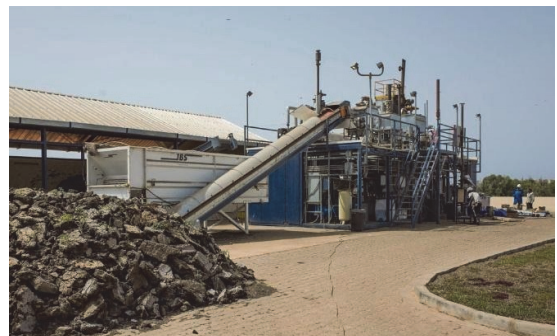
Figure 2.11 The omniprocessor faecal sludge treatment system in operation in Dakar, Senegal (photos: UKZN PRG and Sedron Technologies).
