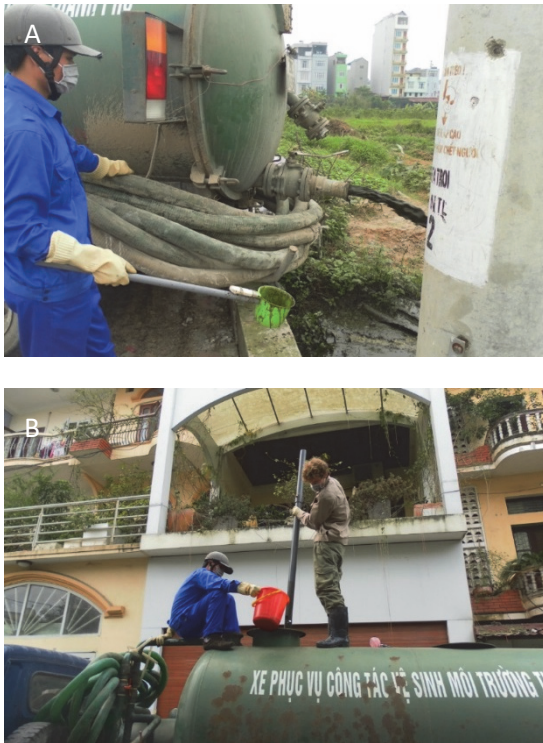
Figure 3.19 A) collecting grab samples from the truck discharge valve to make a composite sample, and B) collecting a core sample from a truck access port with a 180 cm length PVC core sampling device with a 5 cm internal diameter, Hanoi, Vietnam (photos: Eawag).
