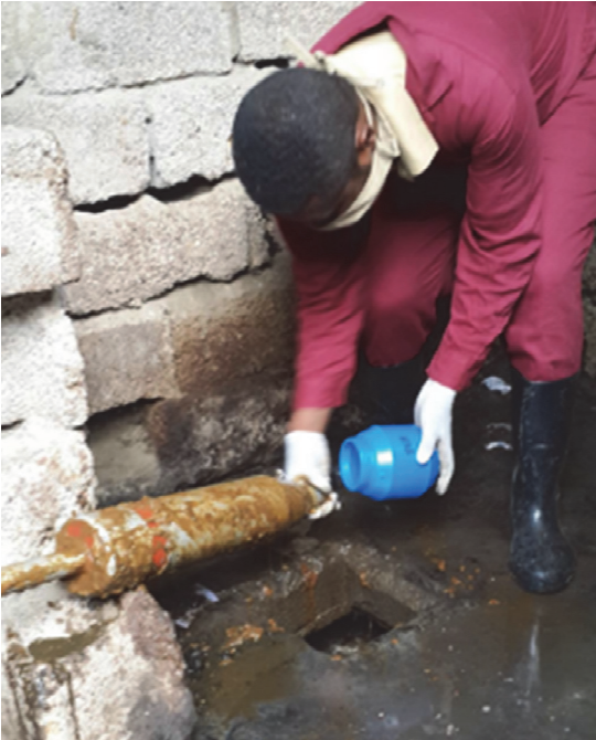
Figure 3.6b Cone-shaped pit-sampling device in use in a study in Ethiopia (photo: Beyene et al. , 2019).
