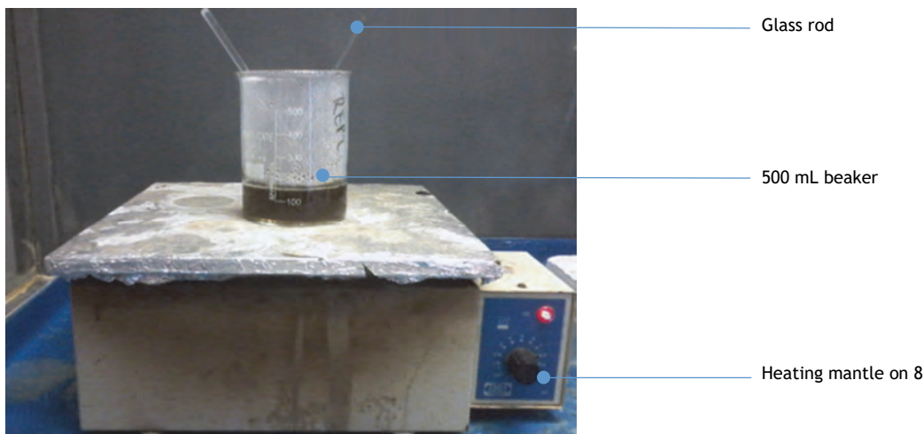
Figure 8.5 Acid-base digestion setup (photo: UKZN PRG).
