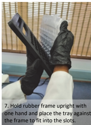
Figure 8.21 Quanti-Tray 200 total coliforms and E. coli procedure (source: UKZN PRG).
