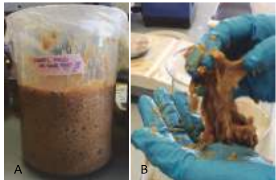
Figure 7.2 Synthetic faeces containing 30 wt % of the solids content baker's yeast. Photo A shows the mixture after standing at room temperature for 1.5 hours and photo B shows a sample of the mixture.
