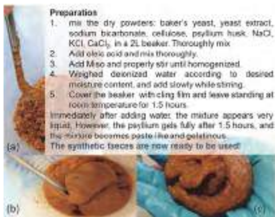
Figure 7.5 Procedure for preparation of synthetic faeces; (a) mixture of synthetic faeces prior to addition of water; (b and c) mixture of prepared synthetic faeces containing ~80% water (b) prepared mixture after standing for 1.5 hours; (c) structured faeces. Tip: Use wet hands, preferable gloves, because the synthetic faeces contain substantial amount of oil.
