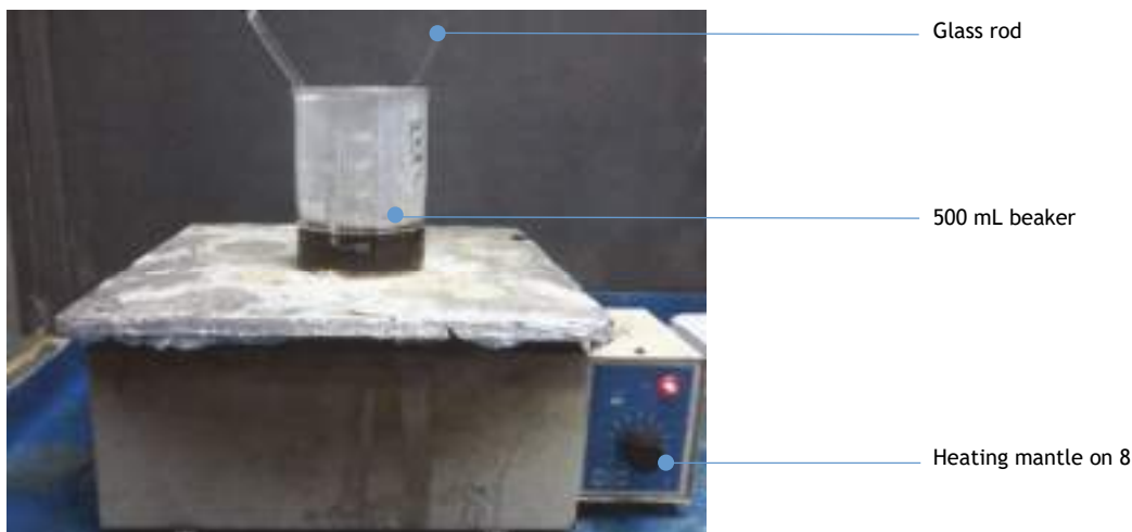
Figure 8.5 Acid-base digestion setup (photo: UKZN PRG).
