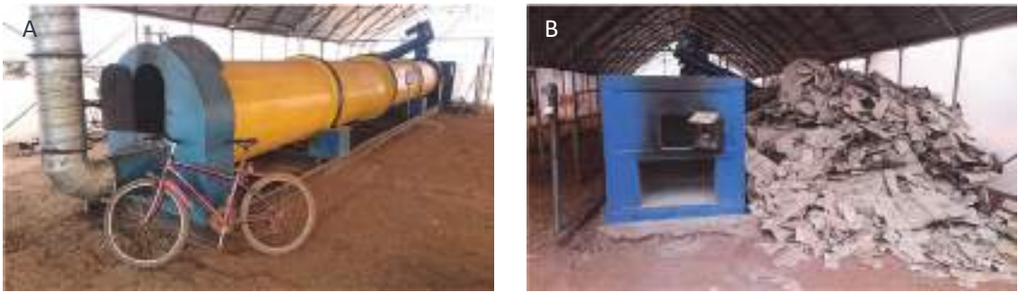
Figure 4.15 A) a rotary convection dryer operated by Pivot, in Kigali, Rwanda and B) waste cardboard is burned in a boiler and the hot gases produced are used as the heat source for drying. The sludge is pre-dried by a solar dryer before entering the convective dryer pictured here (photos: UKZN PRG).
