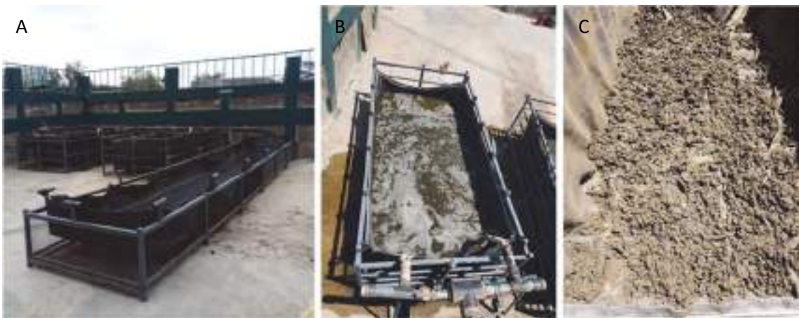
Figure 4.10 A) a geotextile skip setup at the pilot facility; B) a geotextile skip being loaded with conditioned faecal sludge; C) dewatered sludge ready to be unloaded from a geotextile skip (photos: Sanivation).
