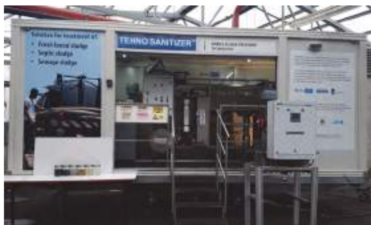
Figure 4.23 A) simplified process flow diagram of the Tehno Sanitizer: (1) sludge intake, (2) sludge pre-treatment, (3) the sludge sterilisation and drying unit, (4) microfiltration, (5) reverse osmosis, and (6) the sludge energy recovery unit, and B) a full-scale Tehno Sanitizer prototype (source: Tehnobiro d.o.o.).
