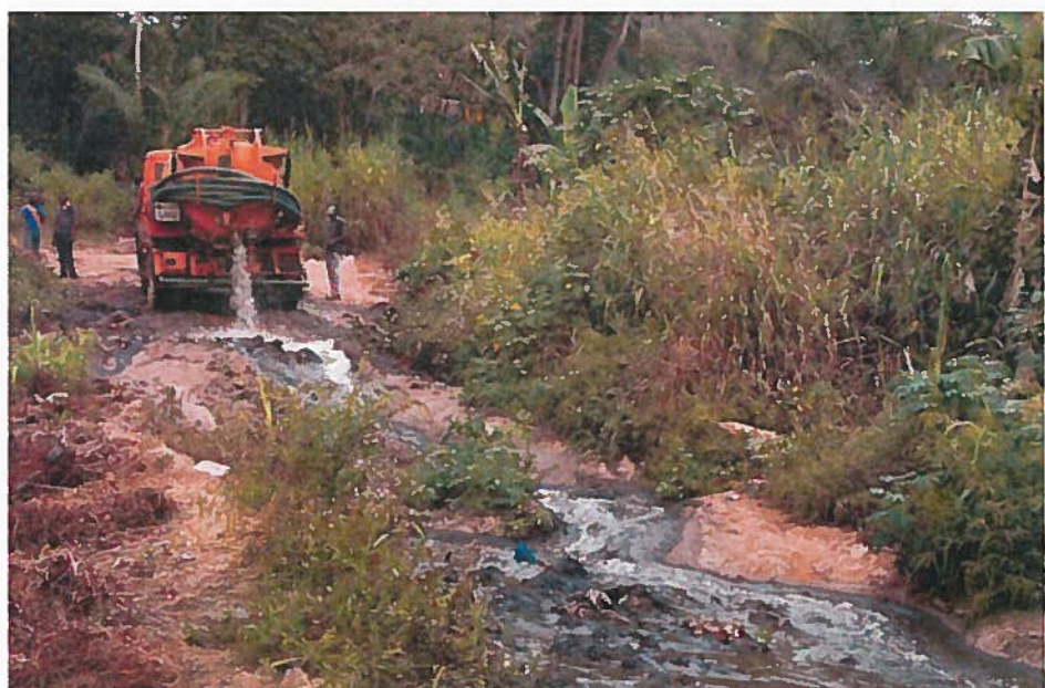
Discharge of faecal sludge into the environment in Yaounde, Cameroon. Credit: Linda Strande.
