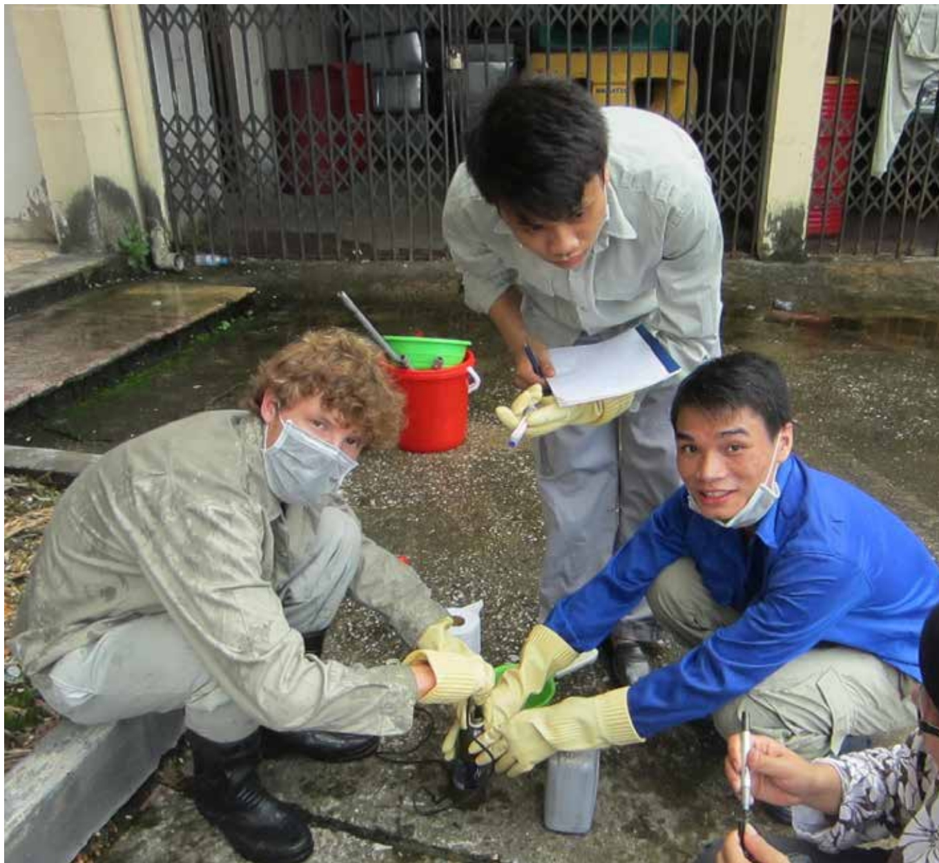
Figure 5: On-site measure of pH and temperature with probes. Photo: Sandec
