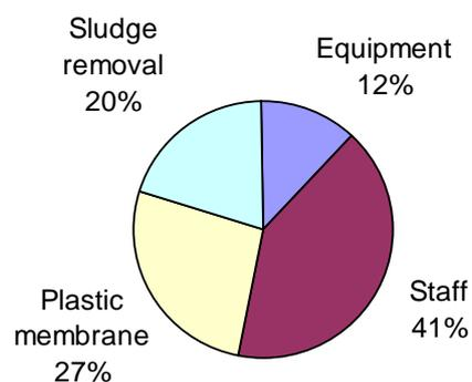
**Figure 3:** Specification of the annual O+M costs of two settling ponds. Total O+M amounts to US\$ 2,960 per year.
