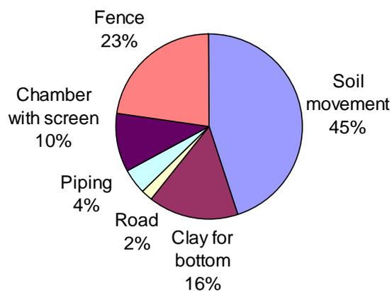
**Figure 2:** Specification of construction costs of two settling ponds. Total costs amount to US\$ 11,580.
