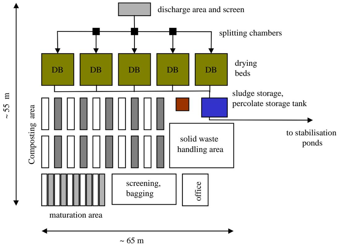
**Figure 11:** Diagram of upscaled co-composting plant (25,000 PE), not to scale.
