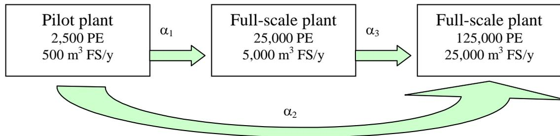
**Figure 13:** Two different ways of upscaling, hence two different parameters  $\alpha$ . Parameter  $\alpha_2$  is a kind of average value of  $\alpha_1$  and  $\alpha_3$ .
