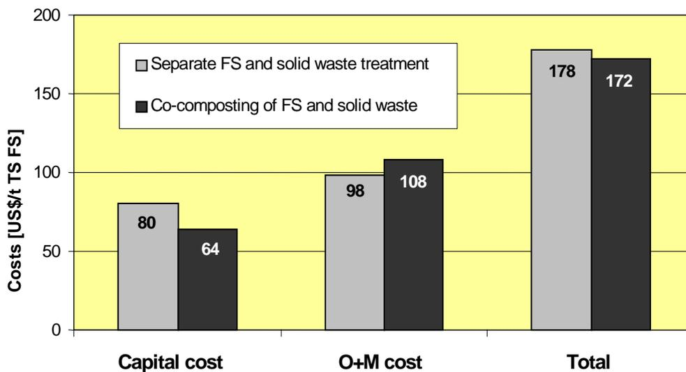
**Figure 19:** Co-composting vs. separate FS and solid waste treatment.
