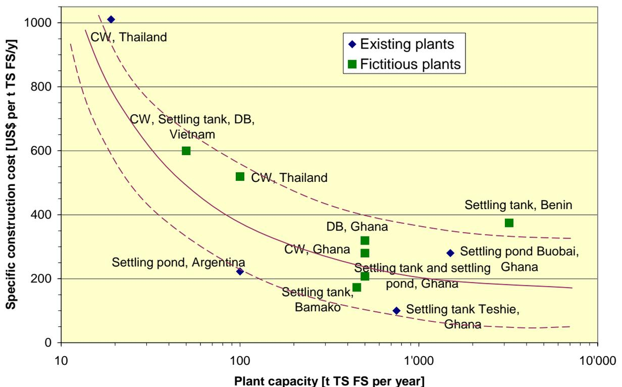
**Figure 20:** FSTP construction costs for different treatment options and countries, including liquid effluent post-treatment, but excluding land costs.
