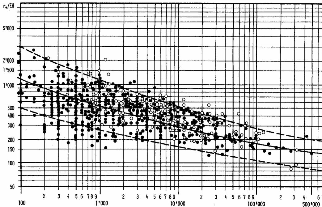
**Figure 9:** Illustration of the economy of scale of WWTP in Switzerland. X-coordinate represents the plant capacity in PE and the y-coordinate the average specific cost in Swiss Fr./PE.(after Maystre 1985).
