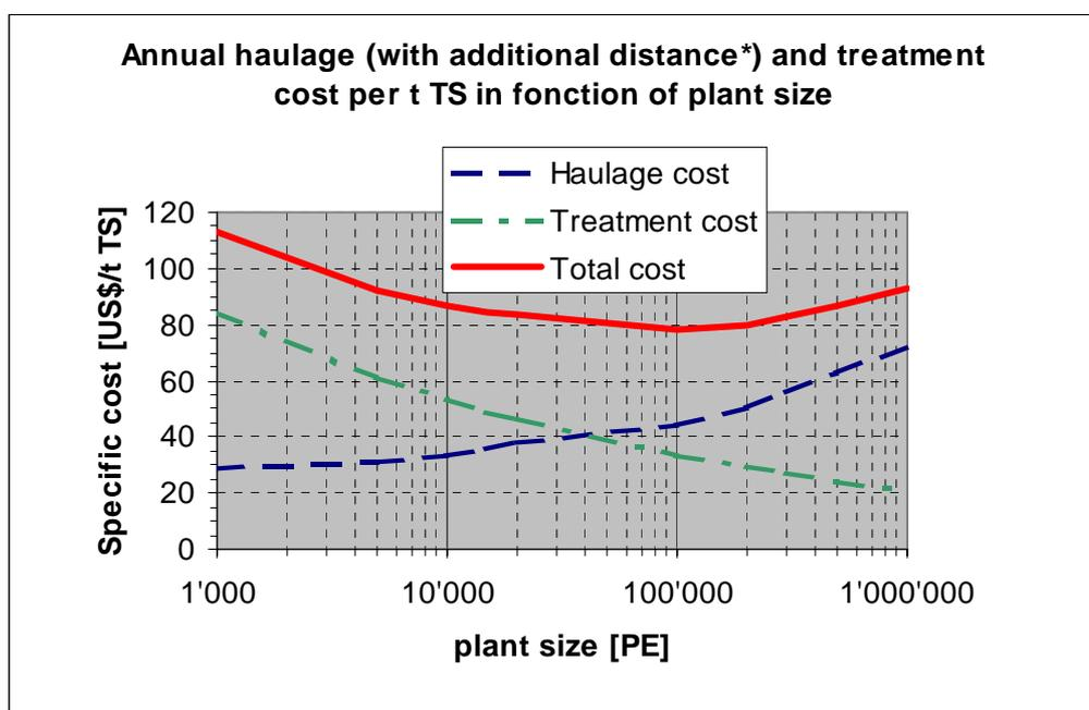
**Figure 10:** Optimal plant size with regard to annualised haulage and capital costs of the treatment plant. (\*Details of the calculation base are given in Paragraph 5.1.3)
