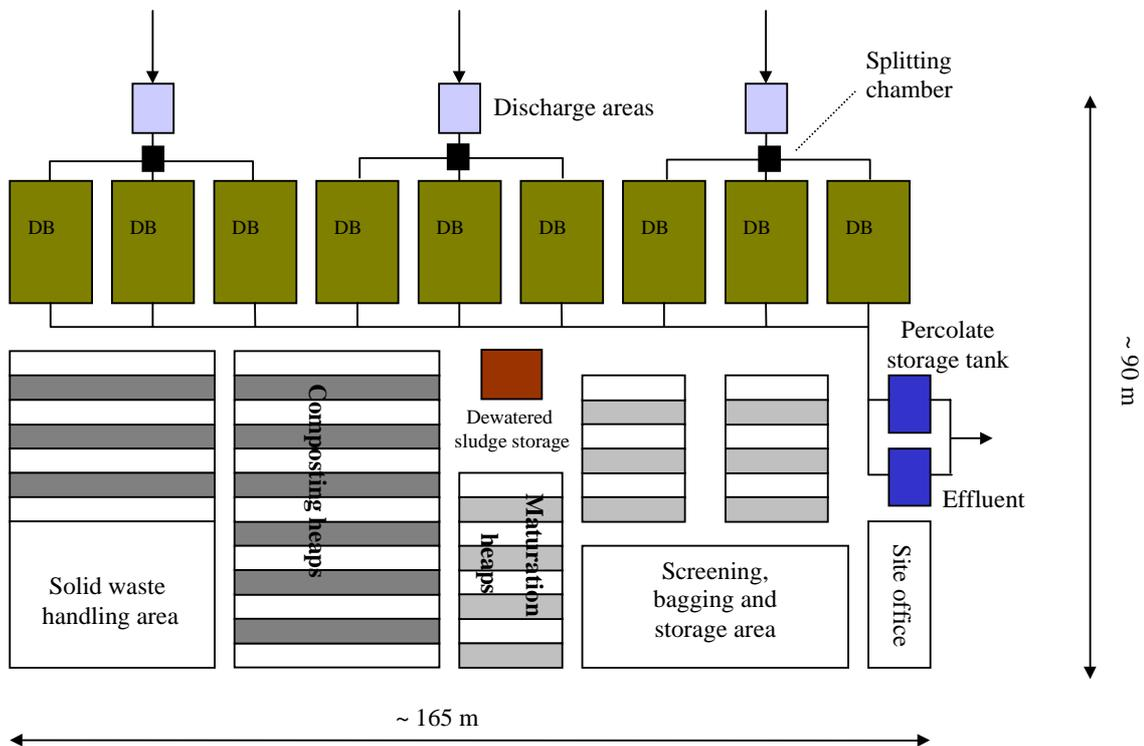
**Figure 12:** Diagram of upscaled plant (125,000 PE), not to scale.
