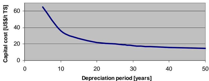
**Figure 7:** Importance of depreciation period in relation to capital costs based on the Buobai full-scale settling pond treatment scheme.
