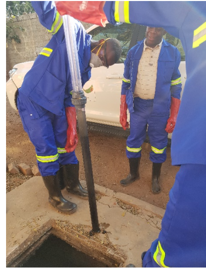
Figure 4: The core sampler with a settled sample from a septic tank.
