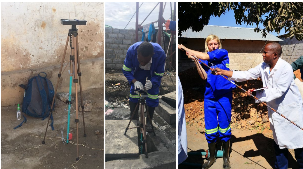
Figure 5: The Volaser in its storage position (left). Volaser measurements being taken in a septic tank (middle). The avalanche probe used to measure depth (right).
