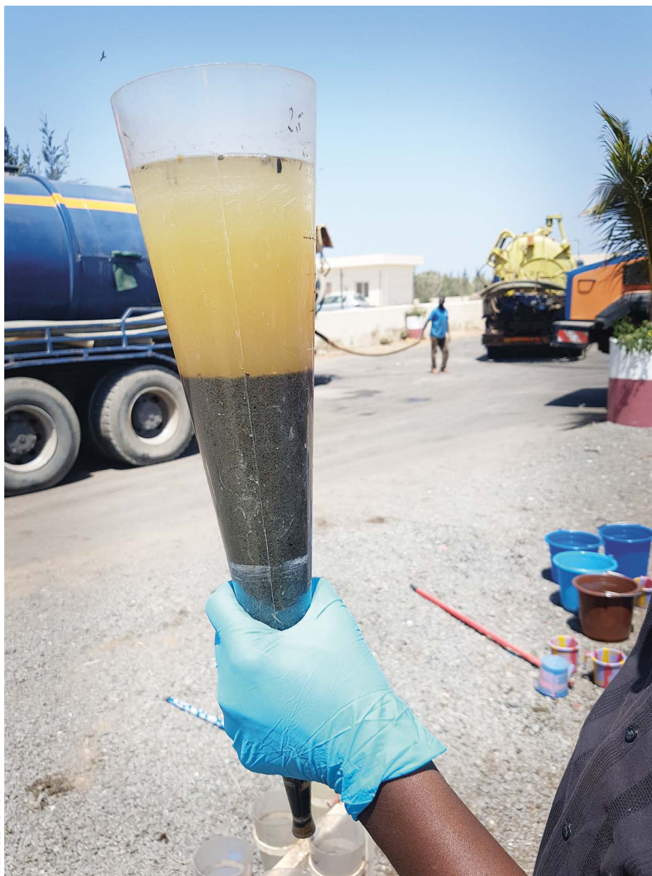
Photo 1: Settling tests on conditioned faecal sludge in Dakar, Senegal.
