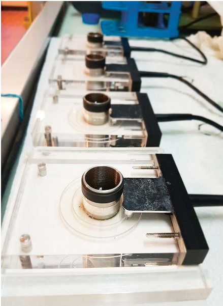
Photo 2: Capillary suction time tests to measure filtration speed of faecal sludge.
