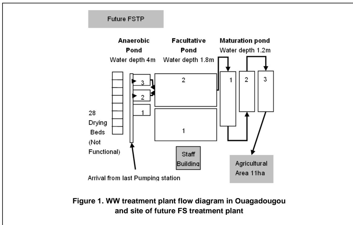
Figure 1. WW treatment plant flow diagram in Ouagadougou and site of future FS treatment plant
