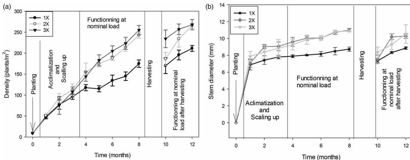
**Figure 1** | (a) Plant density and (b) stem diameter over a one year period with 1X, 2X and 3X weekly loading frequencies of FS at 200 kgTS/m<sup>2</sup>\*year.
