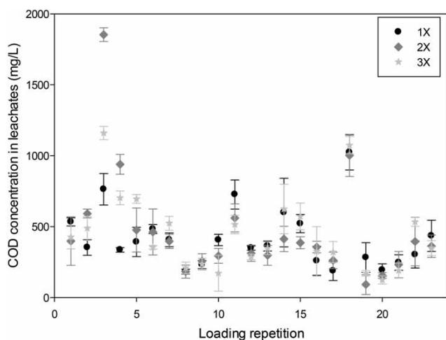
**Figure 2** | COD concentration of leachate over a one year period with 1X, 2X and 3X weekly loading frequencies of FS at 200 kgTS/m<sup>2</sup>\*year.
