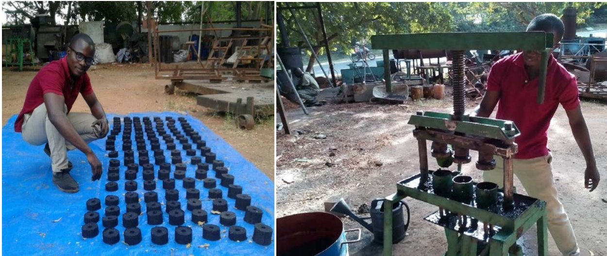
Figure 4: FS char briquettes (left), and Peyam Screw Press machine for making briquettes (right).
