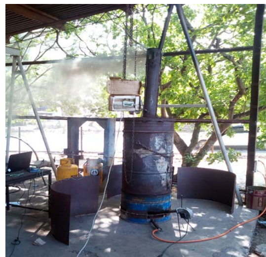
Figure 1: The slow-pyrolysis reactor during an experiment.
