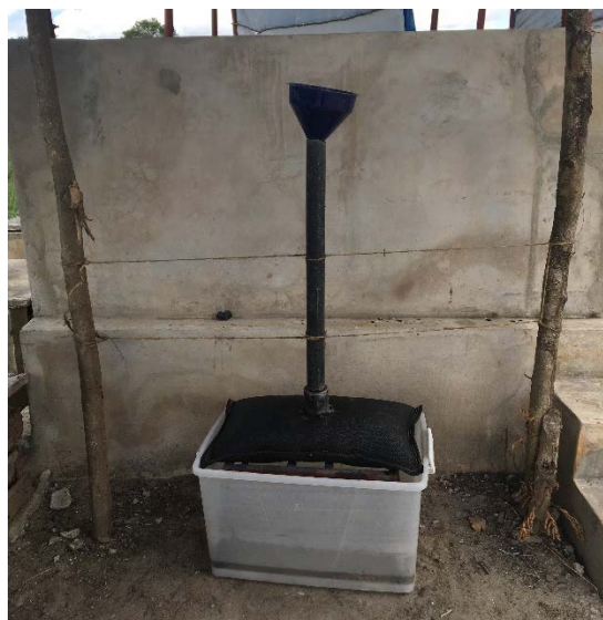
Figure 3: Bench-scale geotube setup
