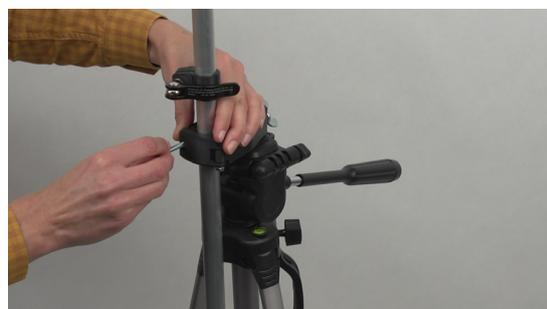
Figure 15: Insert the screw into the hole on the tripod mount clamp.
