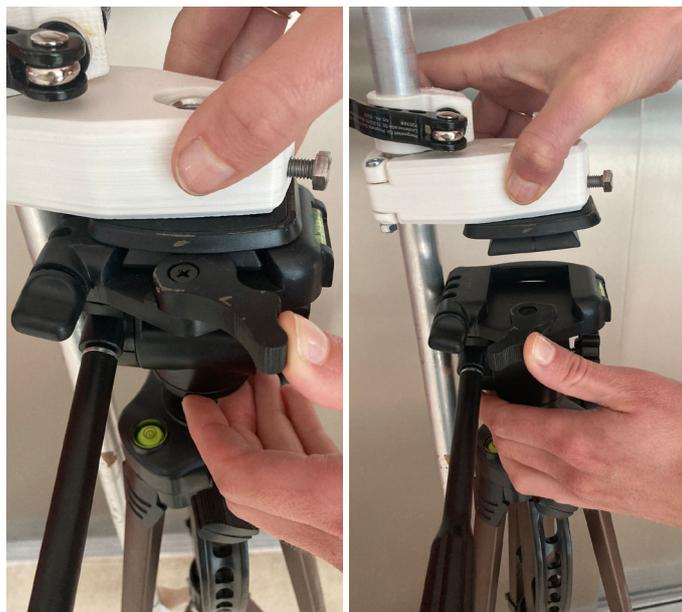
*Figure 32: Some tripod models might have a quick release that allows the metal tube and tripod mount to be easily separated from the tripod.*
