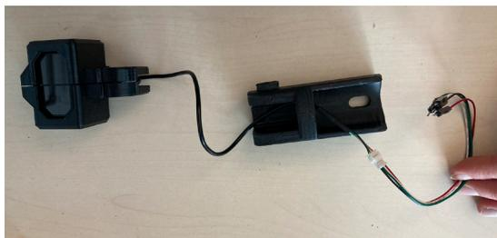
Figure 19: The laser cable winds through the hole in the **12 Laser case connection piece**.
