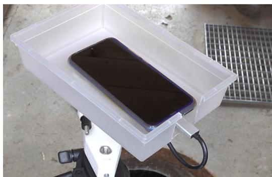
Figure 34: The smartphone needs to be placed horizontally in the protection box and/or smartphone clip.
