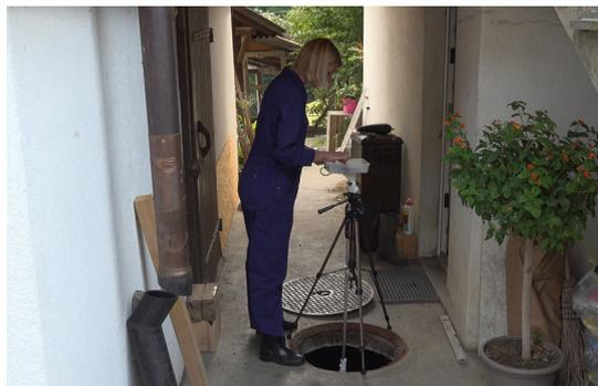
Figure 37: Above: Checking the bubble level on a tripod. Below: The top of the tripod with the protection box should be level while taking a measurement.
