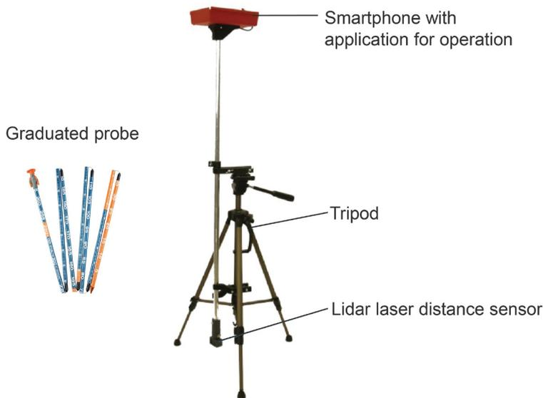
Figure 1: A Volaser device (Andriessen et al., 2023).
