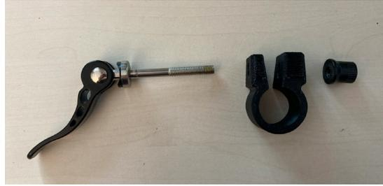
Figure 12: Take the nut off the quick release screw, and stick it through the tube fastener.
