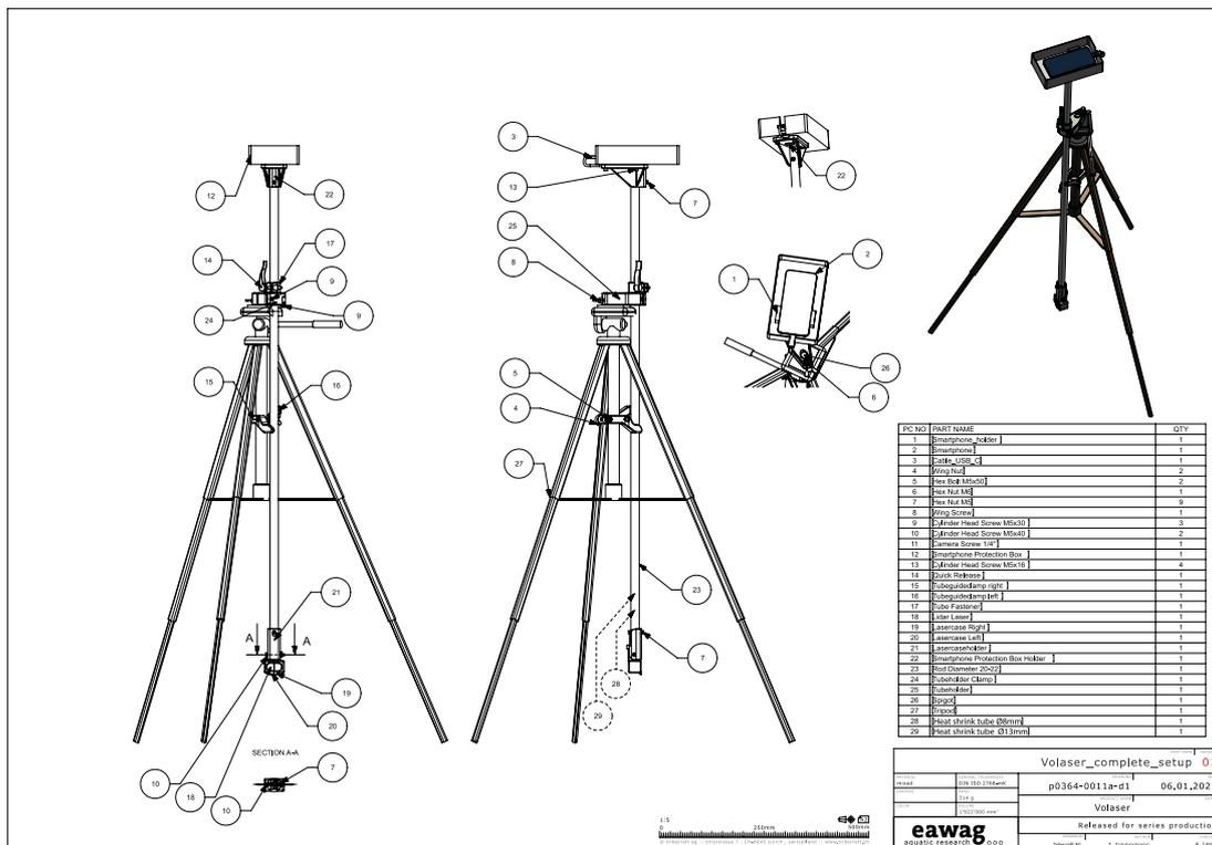
Figure 5: Technical drawing Volaser complete setup. All technical drawings can be found on [www.sandec.ch/volaser](http://www.sandec.ch/volaser) and should be consulted before 3D printing and during assembly.
