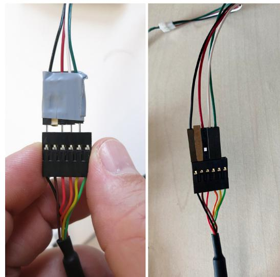
Figure 21: Photo left: The **6 pin FTDI serial TTL connector** (left connector), with the **4 pin connector** to the lidar laser sensor (right connector). Photo right: A cardboard spacer (in brown) to structure the connection between the pins.
