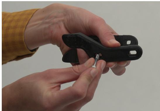
Figure 27: Insert the hex bolts into the designated slots on the Tubeguide - right.
