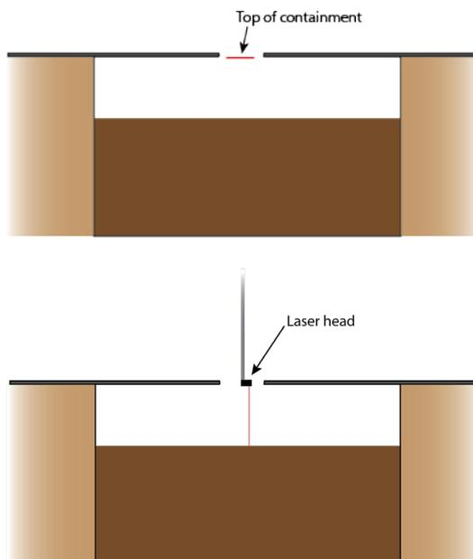
Figure 35: Measure the depth of the containment and the distance to the sludge at the top of the containment.
