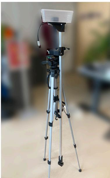
*Figure 31: A Volaser in the storage position: legs fully extended, and in a narrow stance so that the laser does not touch the ground.*
