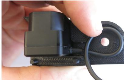
Figure 17: The loop in the laser cable to prevent tension.
