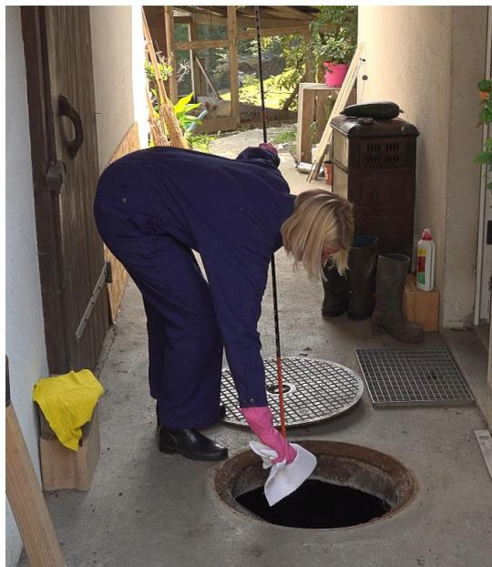
Figure 36: After taking a measurement, clean the probe with a cleaning cloth or sponge.
