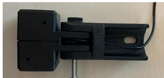
Figure 20: Connect the laser case connection piece to the laser case with a 40mm M5 screw. Make sure that the cable is not in front of the screw hole.
