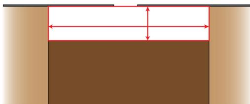
Figure 2: The Volaser uses the area and distance to the sludge layer to calculate the empty volume inside a containment.
