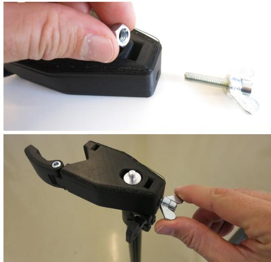
Figure 10: Above: Put a ②③ **Hex nut M6** in the rectangular opening on the narrow part of the tripod mount. Below: Insert the wing screw on the narrow end of the tripod mount and tighten it.
