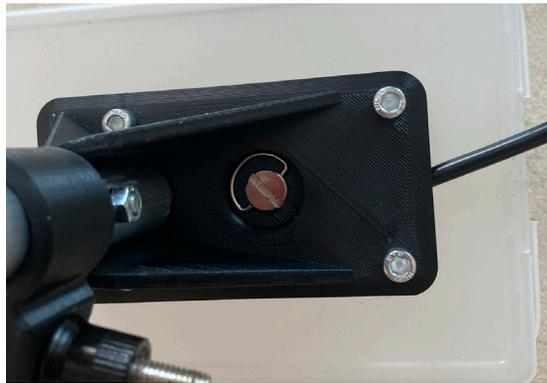
Figure 26: Inserting the quick release screw into the designated slot on the protection box base.
