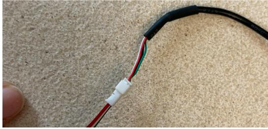
Figure 16: Connect the white JST connectors that come with the **11 Lidar laser**.
