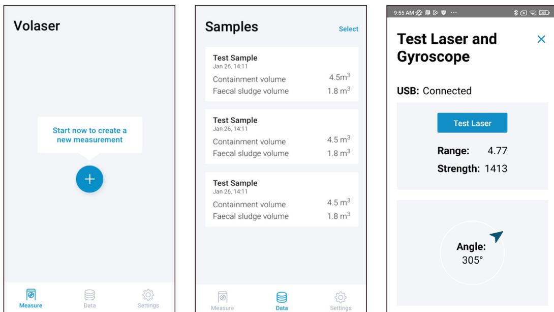
Figure 30: The Volaser smartphone application interface. Left: The 'Measure' tab. Middle: The 'Data' tab. Right: the 'Test Laser and Gyroscope' page.
