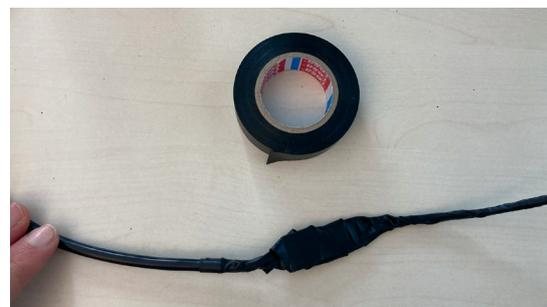
Figure 22: The connector should be securely wrapped in electrical tape.
