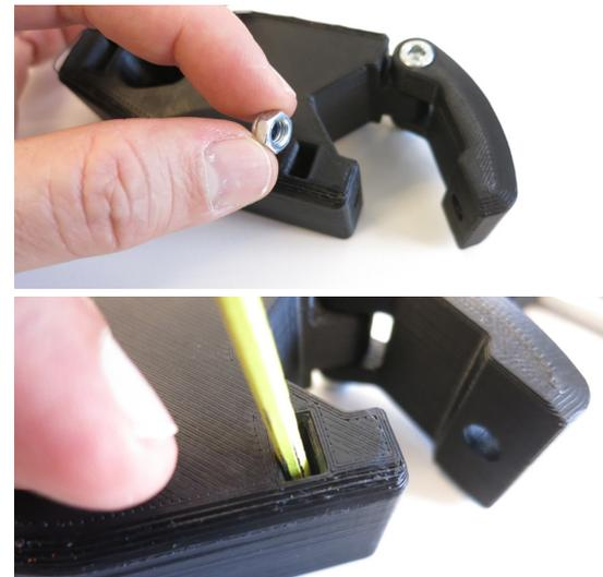
Figure 14: Above: Insert a M5 nut into the last hole on the tripod mount. Below: You might need to push it down.
