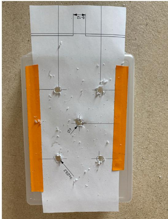
Figure 24: Use a print out of the protection box technical drawing to help place the position of the drill holes
