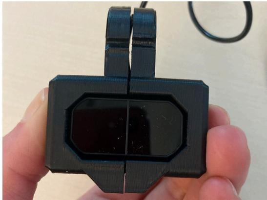
Figure 18: Close both sides of the laser case so that the case surrounds the laser.
