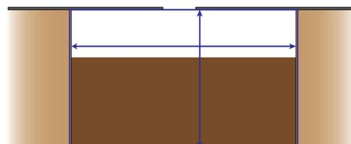
Figure 3: The depth of the containment is measured with a probe. The Volaser then calculates the total containment volume as  $area \times depth$ .
