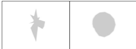
Figure 40: An example of an erroneous measurement of a round pit (left) versus a correct measurement (right).
