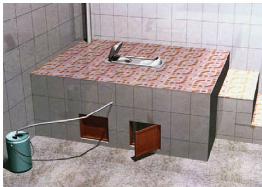
Figure 8.1: Urine-diverting dry toilets built in Zhong Village in the pilot project phase (Source: Lin Jiang 2007, Eawag).
