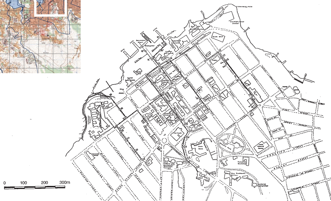
Figure 2.5: Sewerage coverage in Freetown, Sierra Leone (Atkins, 2008) (The continuous black lines indicate installed sewer line.)
