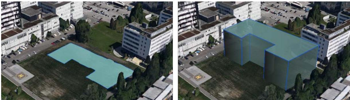
**Figure 8** left: Polygon clamped to the ground (default); right: 3D polygon
