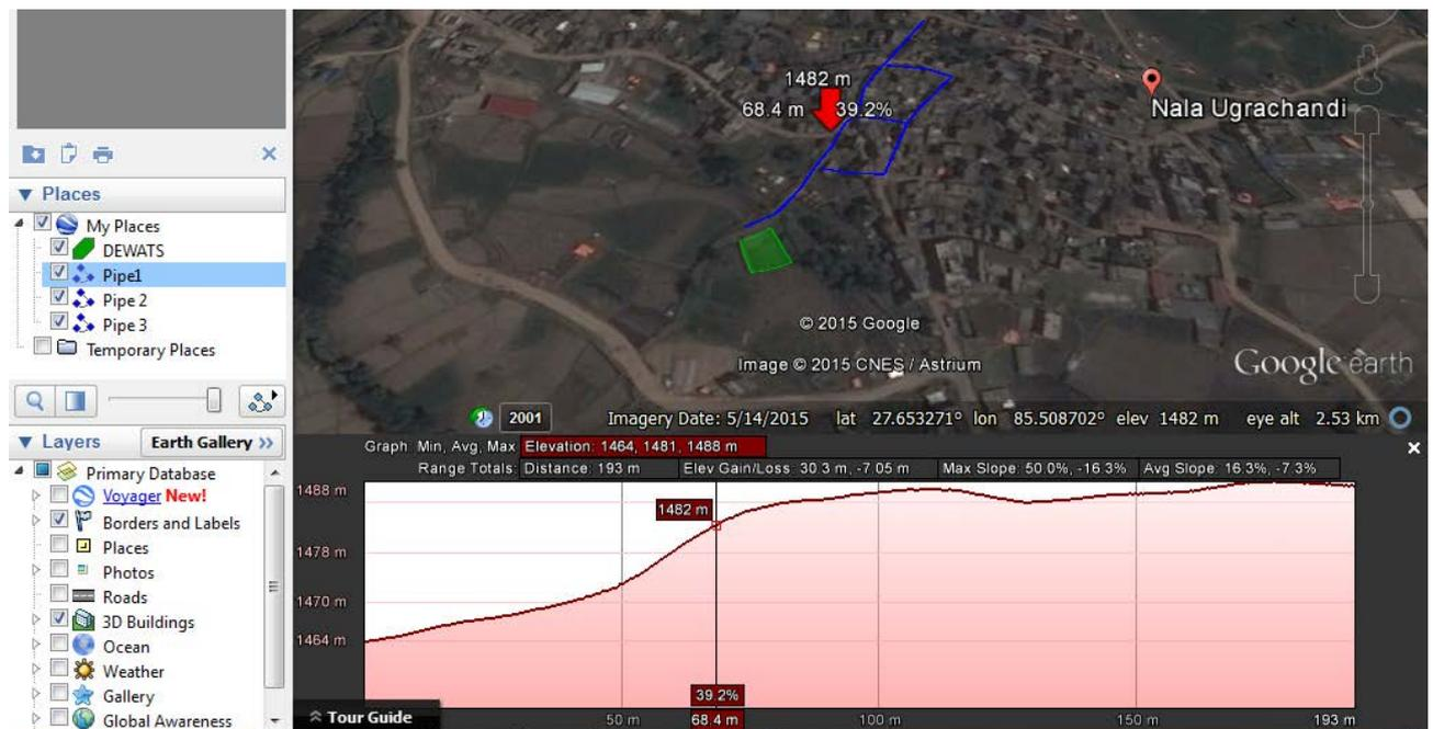
Figure 10 Rough draft of a sanitation system with an elevation profile of a selected sewer pipe.
