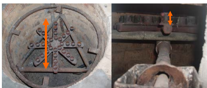
Figure 25: Gas burner (left: from top, diameter 36 cm, right: view at the cylinders surrounding each hole, height 2 cm)
