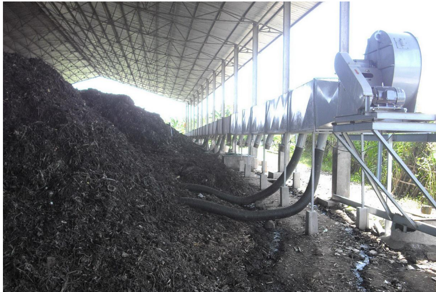
Figure 25 Composting windrows with forced aeration showing blowers and tubes, source (Küper, 2011).
