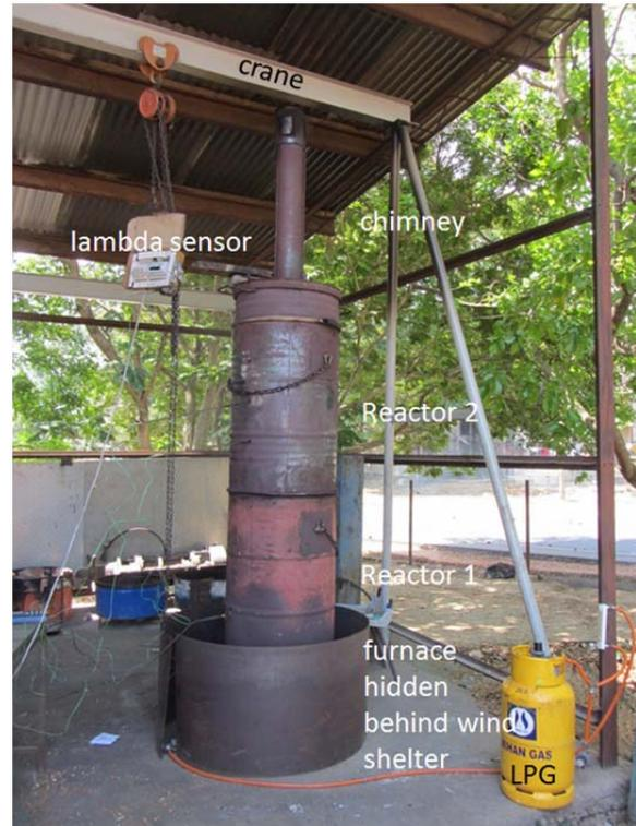
Figure 15: whole new reactor system
