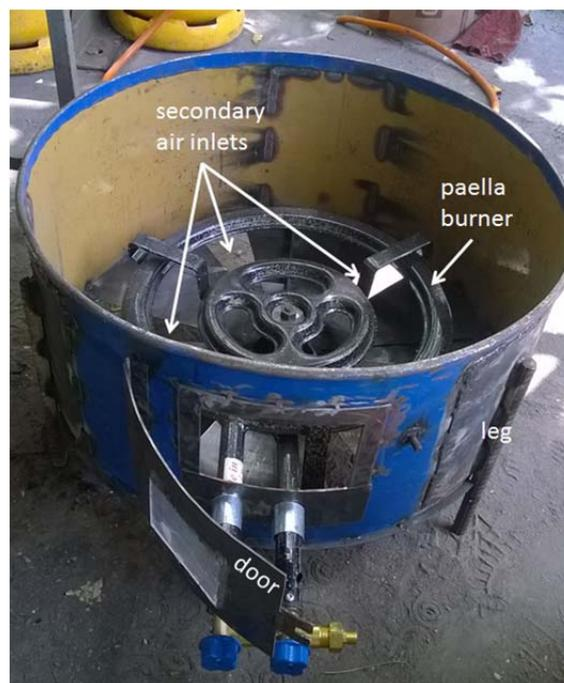
Figure 16: furnace with paella burner
