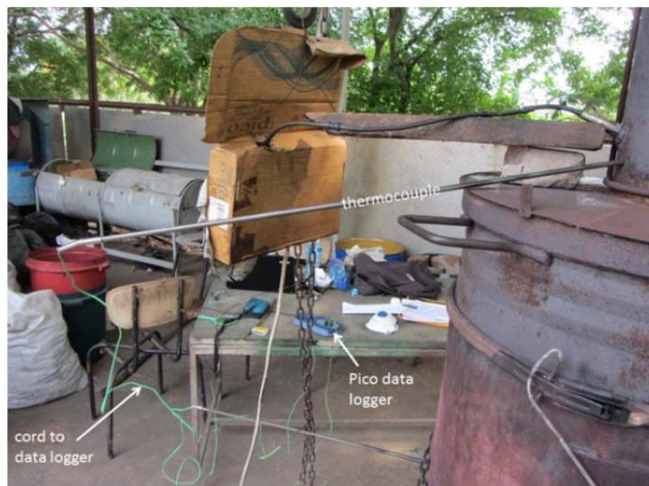
Figure 6: thermocouple installed and connected to the data logger
