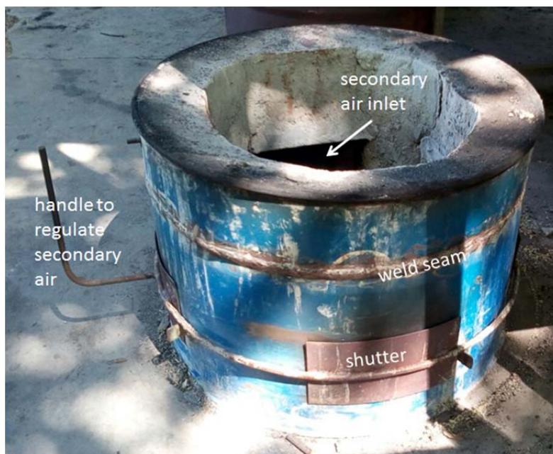
Figure 17: final version of the furnace
