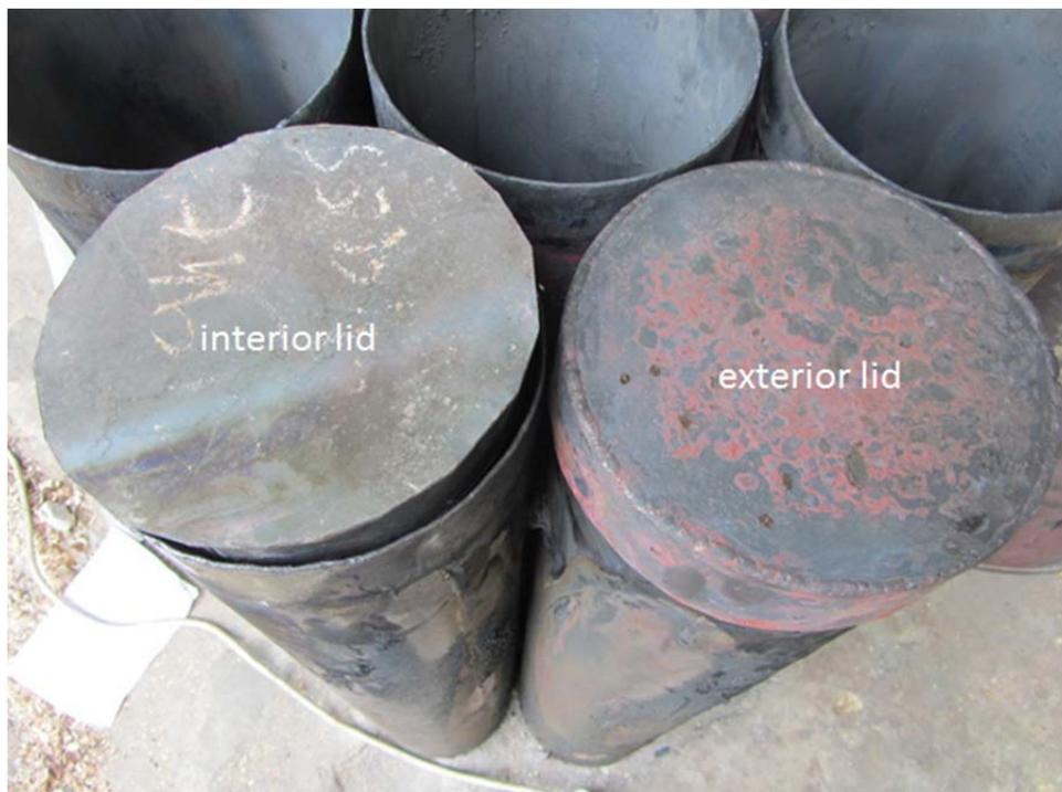
Figure 4: the two different types of lids
