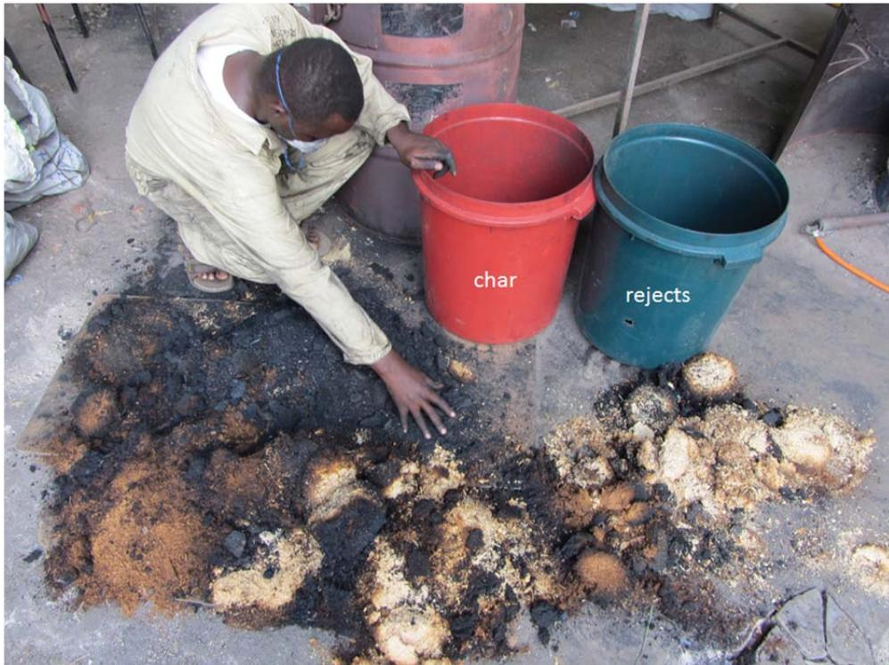
Figure 13: separation of incomplete carbonized feedstock
