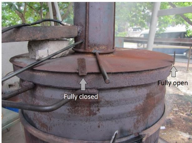
Figure 10: opening position of the chimney in the beginning (almost fully closed)
