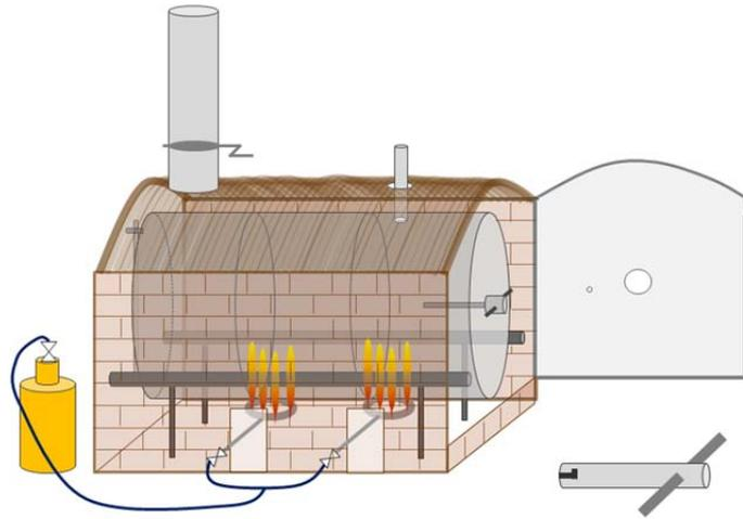
Figure 1: Photo and schematic of first experimental slow pyrolysis unit (Lohri et al., 2015).
