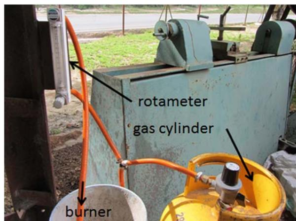
Figure 7: the gas passes through the rotameter from the bottom to the top, proceeding to the burner
