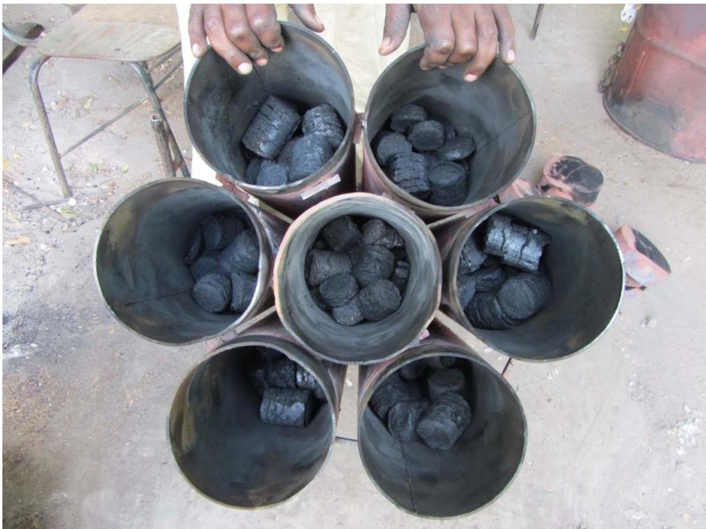
Figure 14: complete pyrolysis of briquettes (experiment ps312) ready to empty
