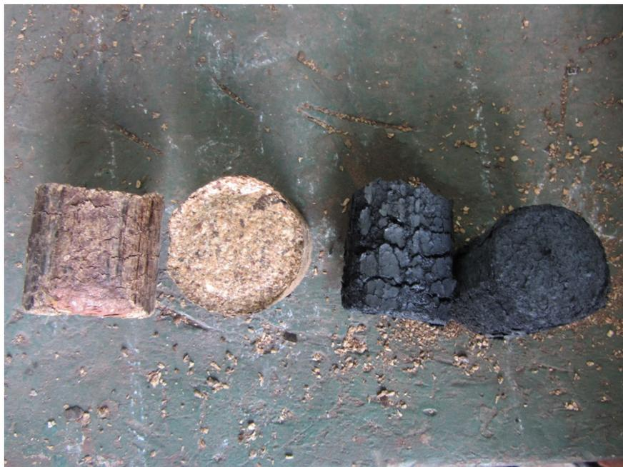
Figure 20: raw vs. carbonized briquette, decrease in diameter and increase in length
