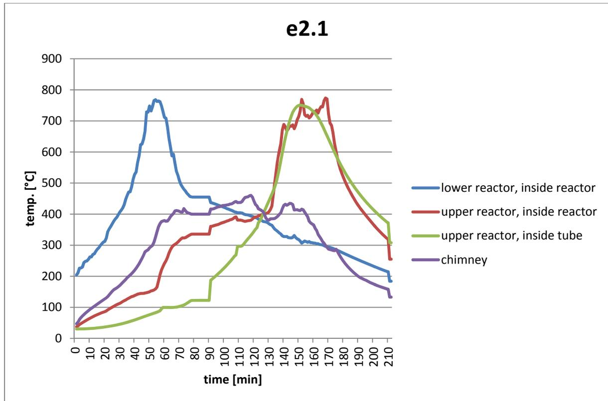
Figure 21: temperature profiles of experiment e2.1
