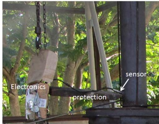
Figure 5: lambda sensor with protection and electronics
