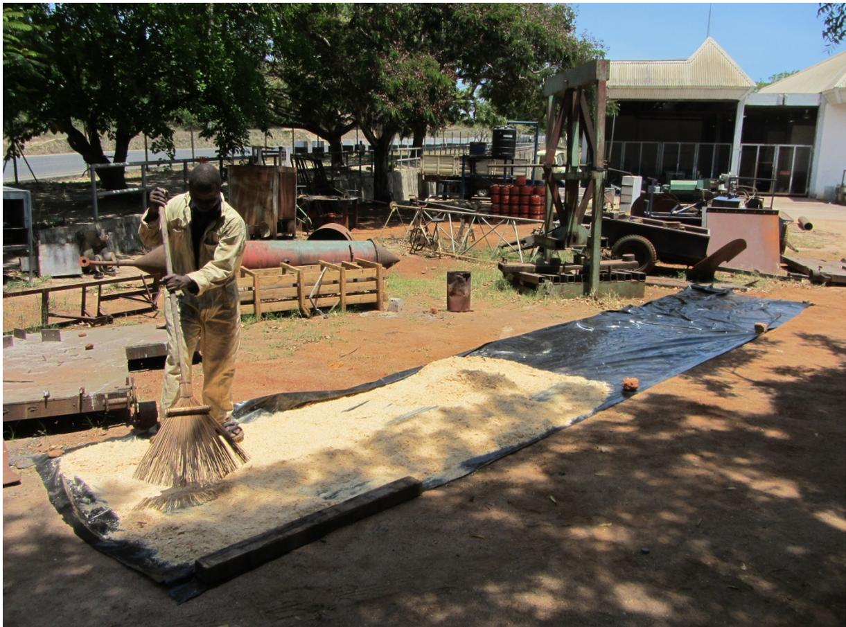
Figure 8: drying of sawdust
