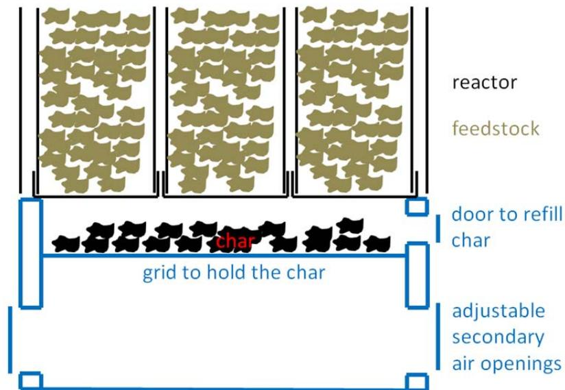
Figure 28: furnace fired with char
