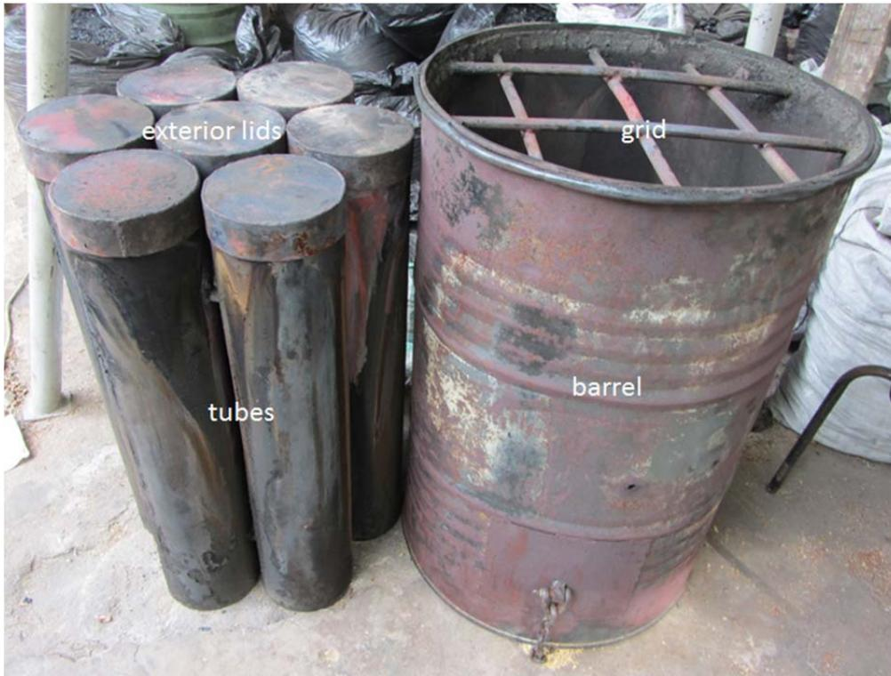
Figure 3: components of Reactor 1
