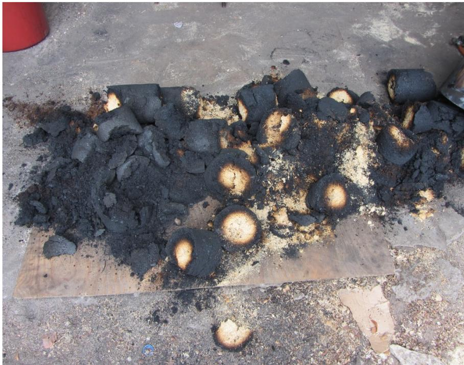
**Figure 24: incomplete pyrolysis (experiment mc212)**
