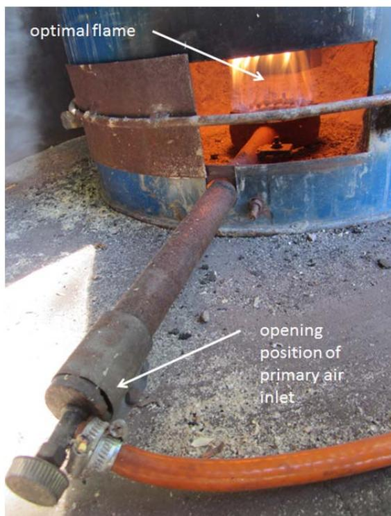
Figure 12: opening position of the primary air inlet and optimal flame
