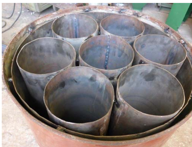
Figure 3: Close-up of the open barrel, the slightly smaller cylinder and the 7 pipes in the cylinder.
