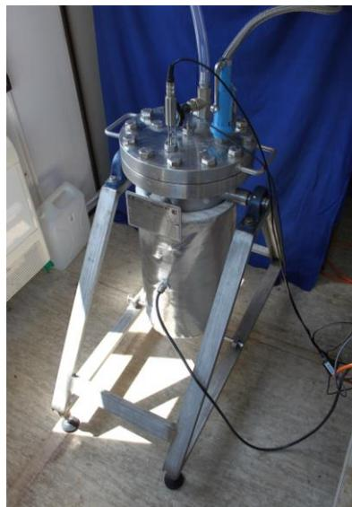
**Fig. 1:** Schematic and photo of the HTC reactor used [29] with inner temperature and pressure measurements, external thermocouples, and drain and overpressure valve placed on the lid
