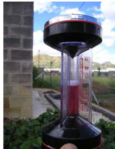
**Picture 21:** Testoryt device to measure the CO<sub>2</sub>-content of gas. CO<sub>2</sub> gets absorbed by the liquid. Thus the volume of the liquid increases correspondingly.
