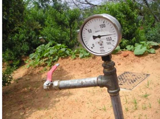
**Picture 2:** Gas tightness is first controlled in the gas piping system that goes from the digester outlet to the end users (for example stove).
