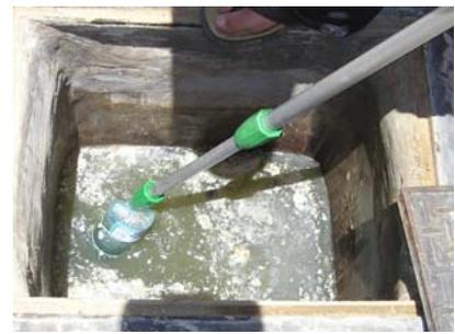
**Picture 9:** Sampling effluent from dome outlet (24.11.2008).
