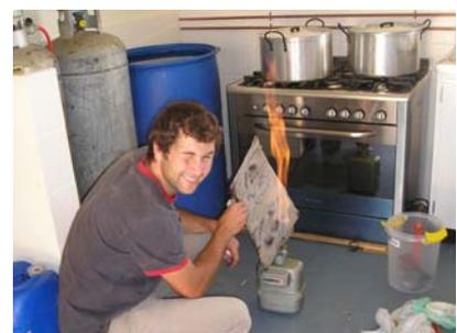
**Picture 12:** Gas measurement; biogas is flamed. Plastic pipe is protected (4.12.2008)
