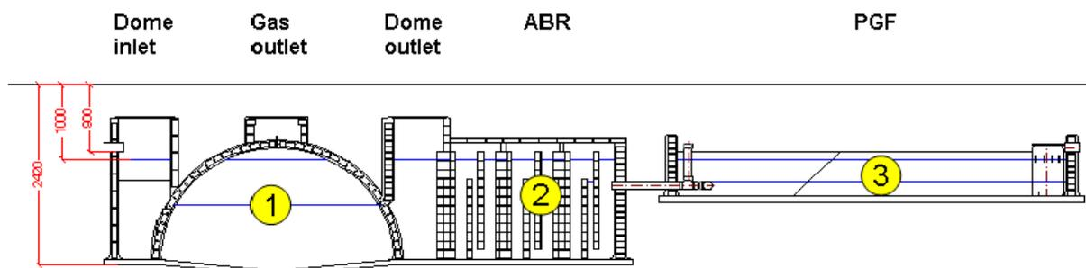
**Figure 2:** Scheme of DEWATS-Biogas-System of TED-Borda. The basic buildup consists of a digester (1), an anaerobic baffled reactor (ABR,2) and an planted gravel filter (PGF,3).
