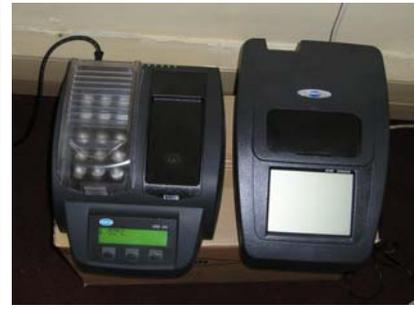
**Picture 12:** Test cube heater (on the left) and photospectro-meter (on the right).
