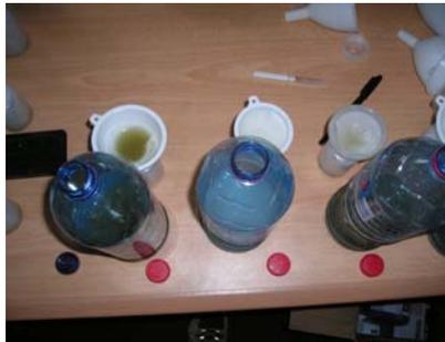
**Picture 10:** Filtering process. Duration depends on solid content within effluent (filters can clog).
