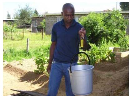
**Picture 24:** The feedstock material is weighed with a hanging balance before put into the inlet chamber.
