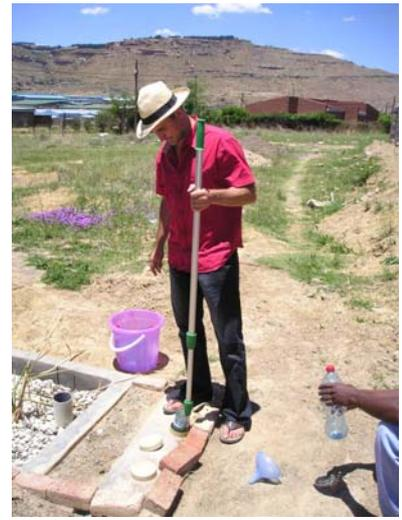
**Picture 18:** Taking effluent samples from ABR (24.11.2008).
