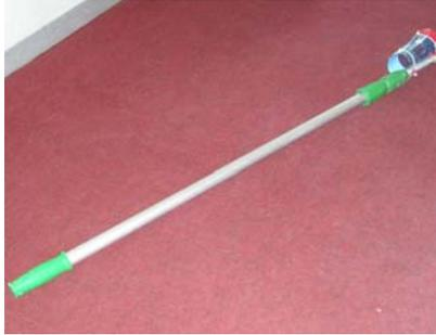
**Picture 1:** Effluent sampling stick. This sticks enables to samples through the tight cover holes of the ABR.
