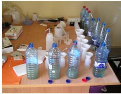
**Picture 5:** Effluent is filtered and stored in small plastic cases.
