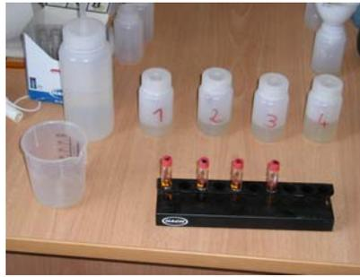
**Picture 11:** Hach Lange test cubes in the front (COD TNT822 and TNT823 were used).
