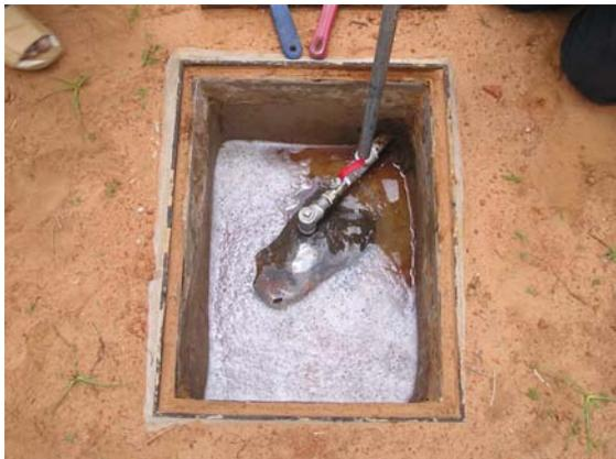
**Picture 3:** Secondly the gas tightness is tested on the top of the digester within the brick chamber. This is done by filling in soap water that enables the identification of leakages (when soap bubbles occur). In order to see any leakage a certain gas pressure has to be build up within the digester.
