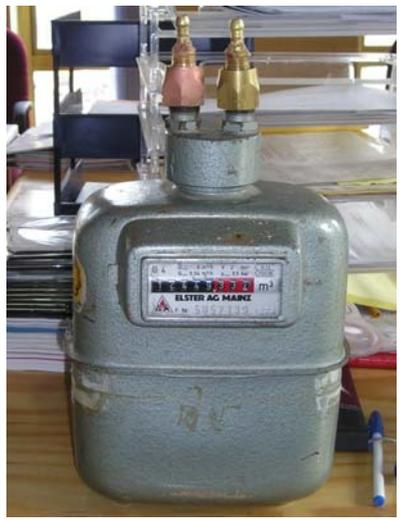
**Picture 20:** Soldered connections on top of the gas meter. This gas meter was used for gas measurements at several plants.
