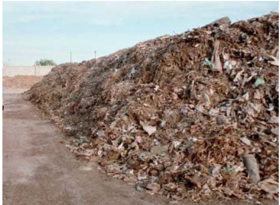
Figure 2: KCDC, elongated heaps (windrows) on sealed composting surface
