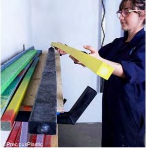
Plastic extrusion is an upcycling technology that converts discarded plastic waste into a continuous plastic filament, which can be further molded into any desired end-product shape.
