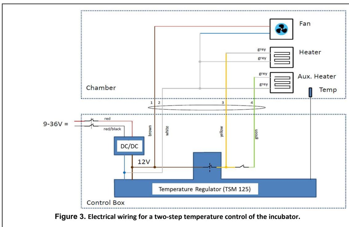
Figure 3. Electrical wiring for a two-step temperature control of the incubator.
