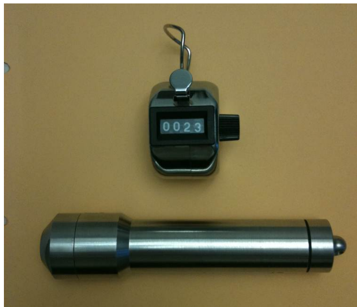
Photograph 1. Tally counter and datalogger
