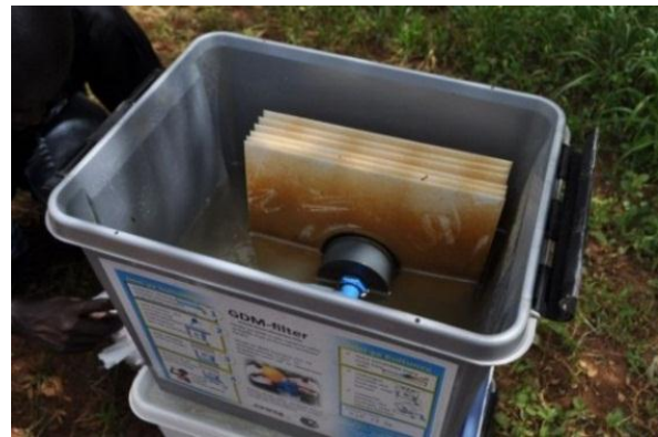
Figure 21 Indication of a red fouling layer on the ultrafiltration membrane.
