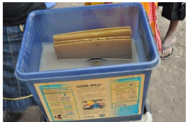
Figure 25 Coating on the ultrafiltration membrane resulting from the use of pond water.
