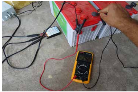
4. Amperage coming out of charge controller (controller to incubator)
