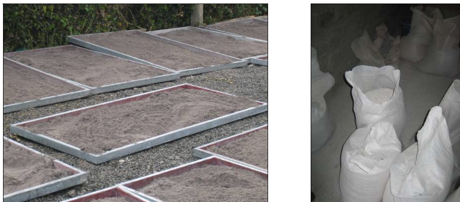
Figure 5-1: Drying the bone char and packed bone char ready for use.
