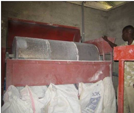
Figure 8-3: Crushing machine with attached sieving units and a separate sieving machine to facilitate and accelerate the sieving process.
