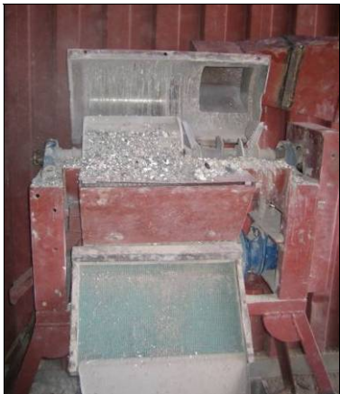
Figure 8-3: Crushing machine with attached sieving units and a separate sieving machine to facilitate and accelerate the sieving process.
