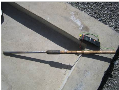
Figure 8-4: Testo 925 to measure the temperature in the furnace. The wood and metal rod protect the delicate wire that transmits the information to the measuring equipment.
