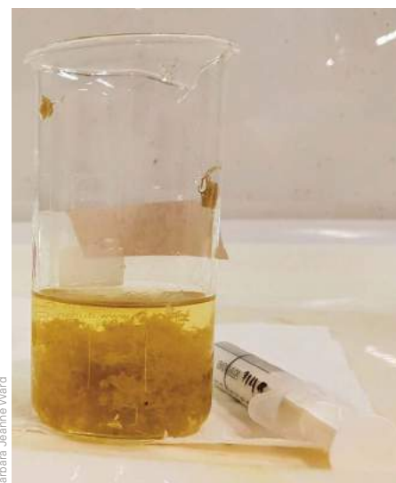
Photo 4: Faecal sludge after conditioning with polymer flocculant. Distinct flocs are visible and the supernatant turbidity is reduced.
