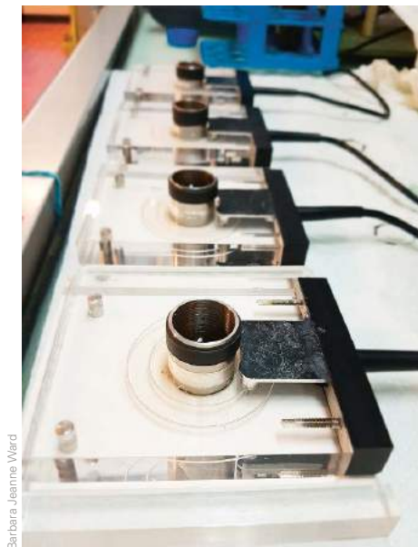
Photo 2: Capillary suction time tests to measure filtration speed of faecal sludge.
